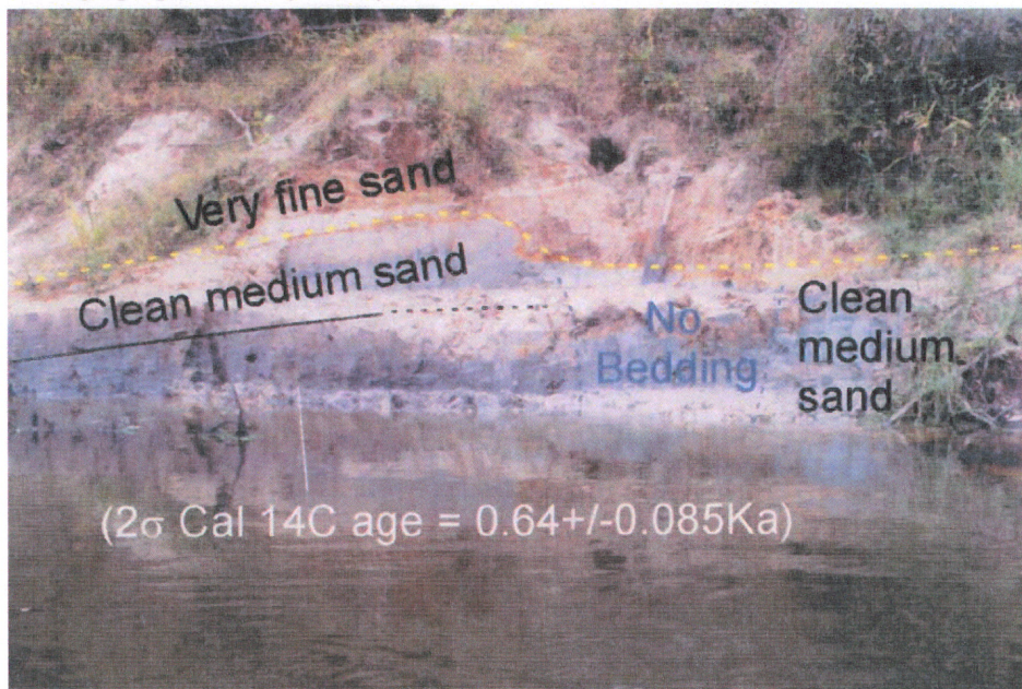
B) Close up view of Holocene sediments involved in folding. Photograph provided by Randy Cox.
