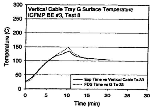
Figure A-54. Thermal environment near Vertical Cable Tray G, ICFMP BE #3, Tests 2 and 8.
