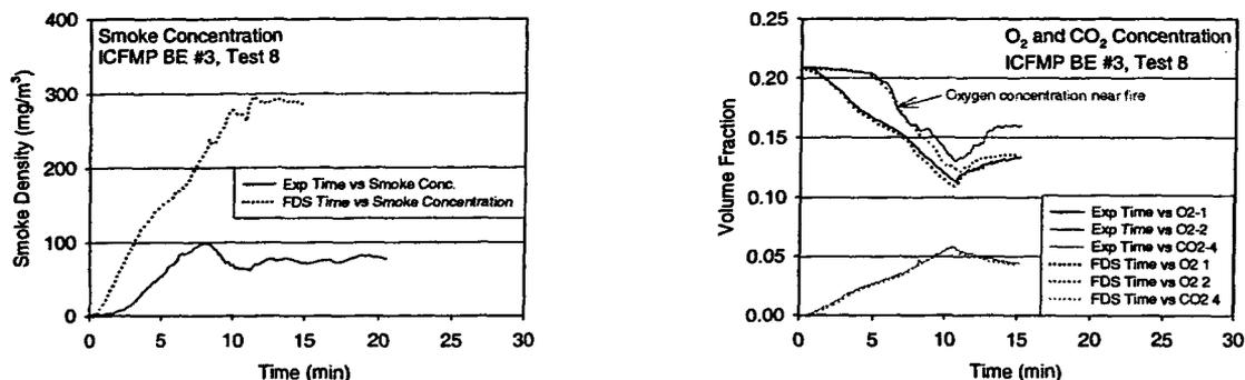
Figure 6-7. Smoke and oxygen concentration, ICFMP BE #3 Test 8.
