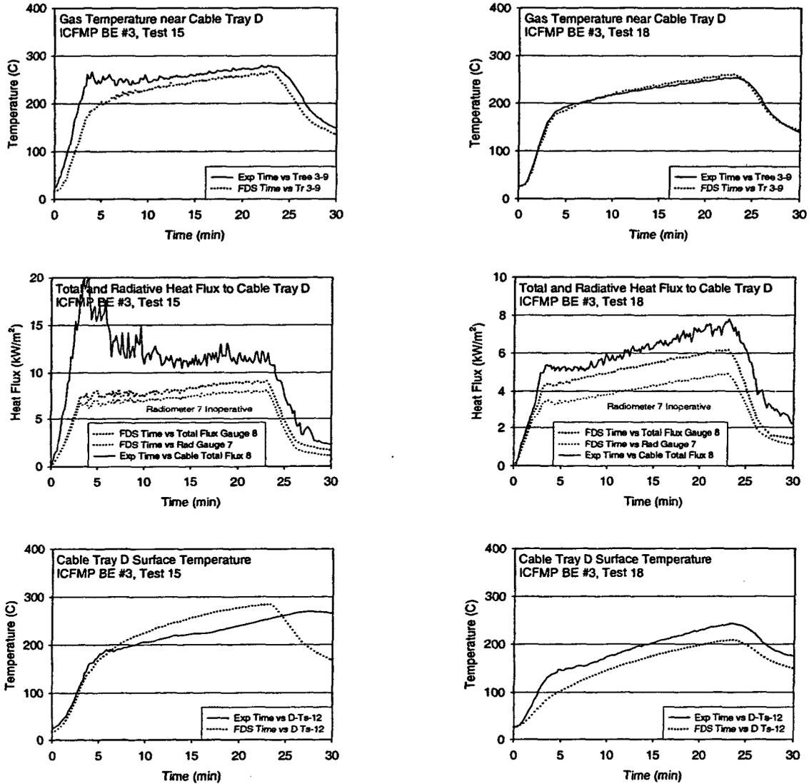
Figure A-45. Thermal environment near Cable Tray D, ICFMP BE #3, Tests 15 and 18.
