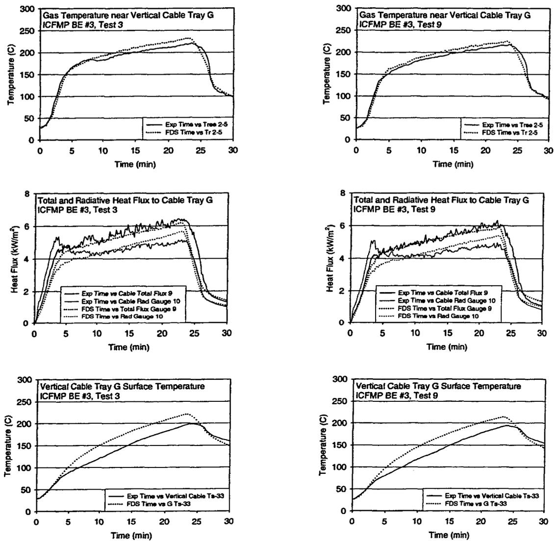
Figure A-57. Thermal environment near Vertical Cable Tray G, ICFMP BE #3, Tests 3 and 9.
