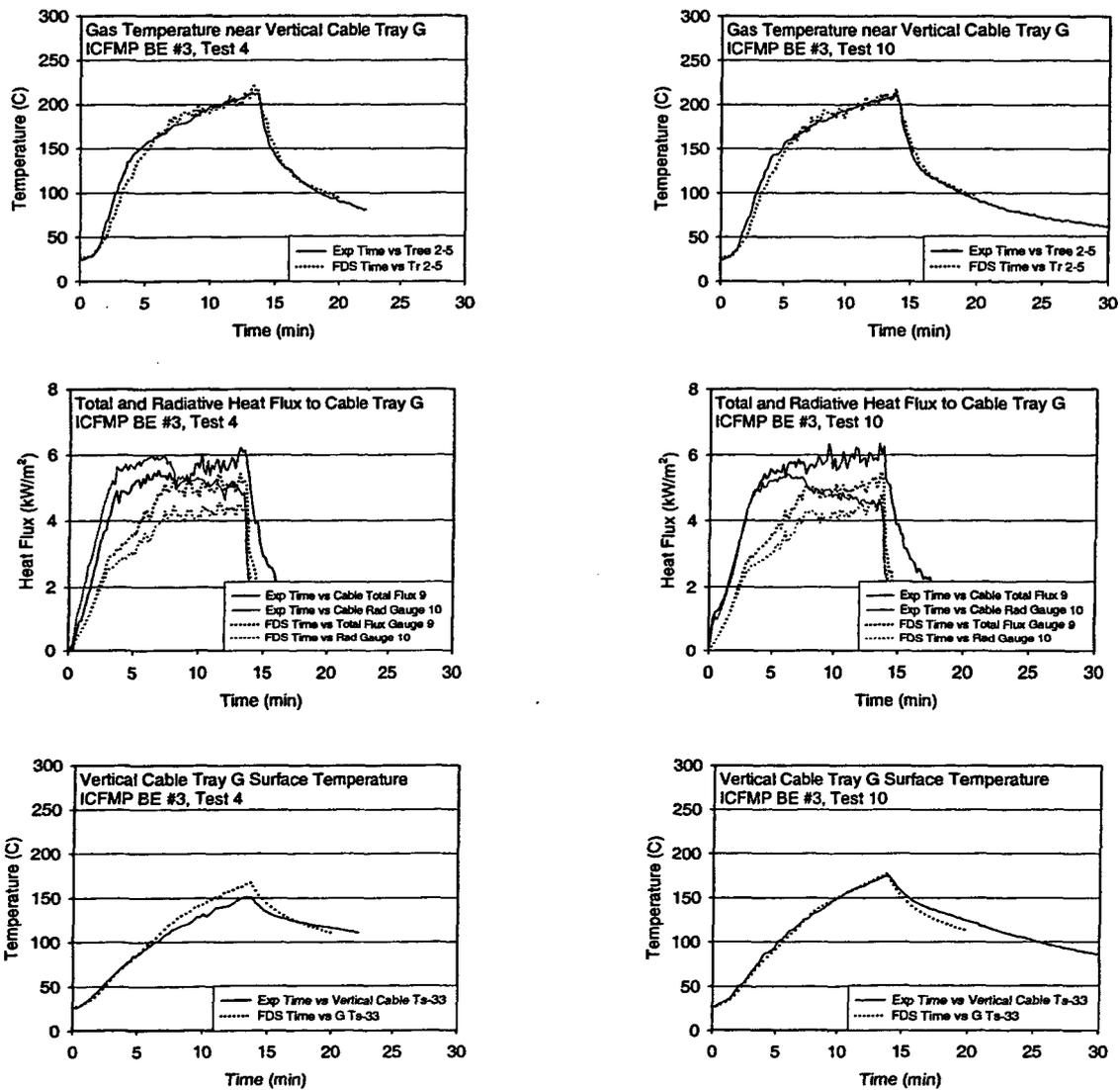
Figure A-55. Thermal environment near Vertical Cable Tray G, ICFMP BE #3, Tests 4 and 10.
