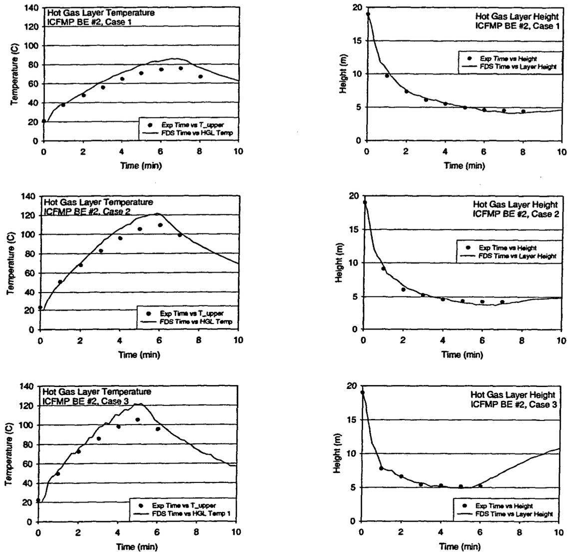
Figure A-2. Hot Gas Layer (HGL) Temperature and Height, ICFMP BE #2.
