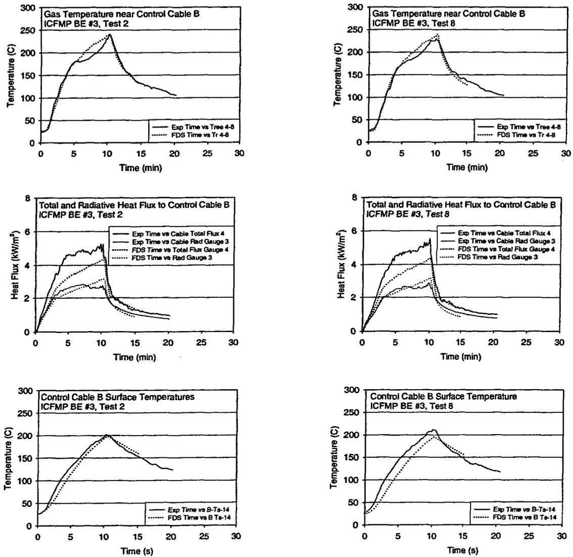
Figure A-33. Thermal environment near Cable B, ICFMP BE #3, Tests 2 and 8.
