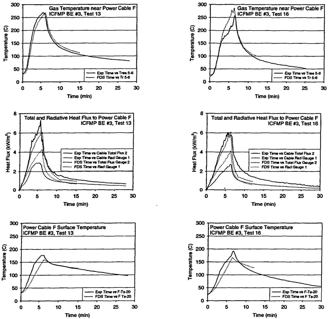
Figure A-49. Thermal environment near Power Cable F, ICFMP BE #3, Tests 13 and 16.
