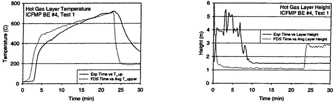
Figure A-9. Hot Gas Layer (HGL) Temperature and Height, ICFMP BE #4, Test 1.
