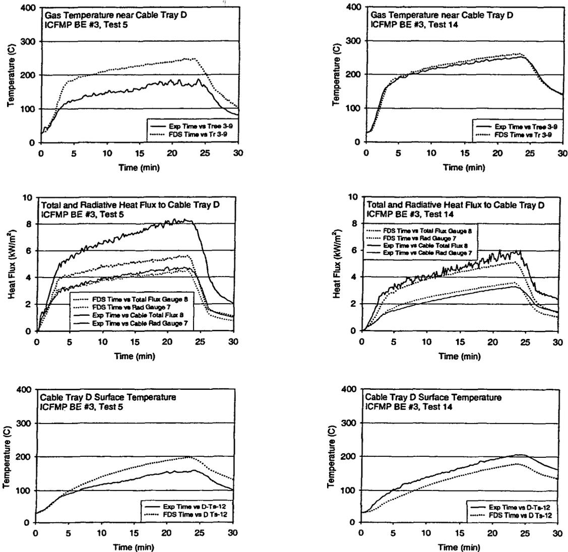
Figure A-44. Thermal environment near Cable Tray D, ICFMP BE #3, Tests 5 and 14.
