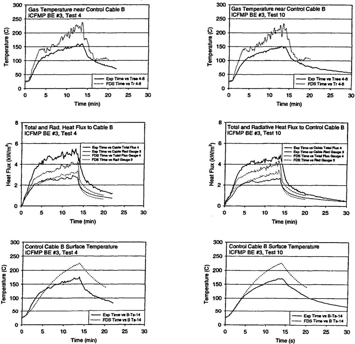
Figure A-34. Thermal environment near Cable B, ICFMP BE #3, Tests 4 and 10. Note the influence of the fan on the gas and surface temperatures.
