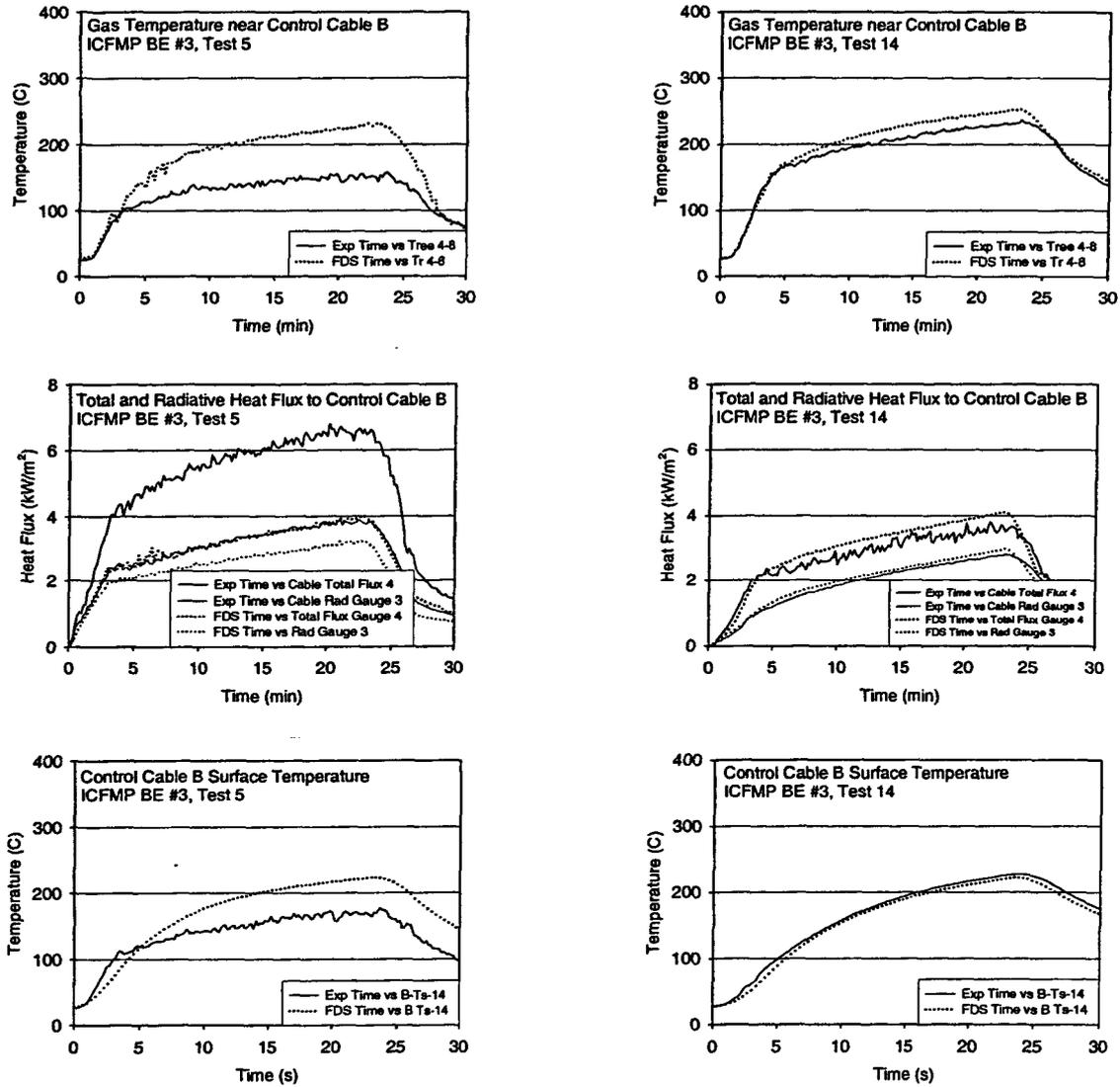
Figure A-37. Thermal environment near Cable B, ICFMP BE #3, Tests 5 and 14. Note the influence of the fan in Test 5.
