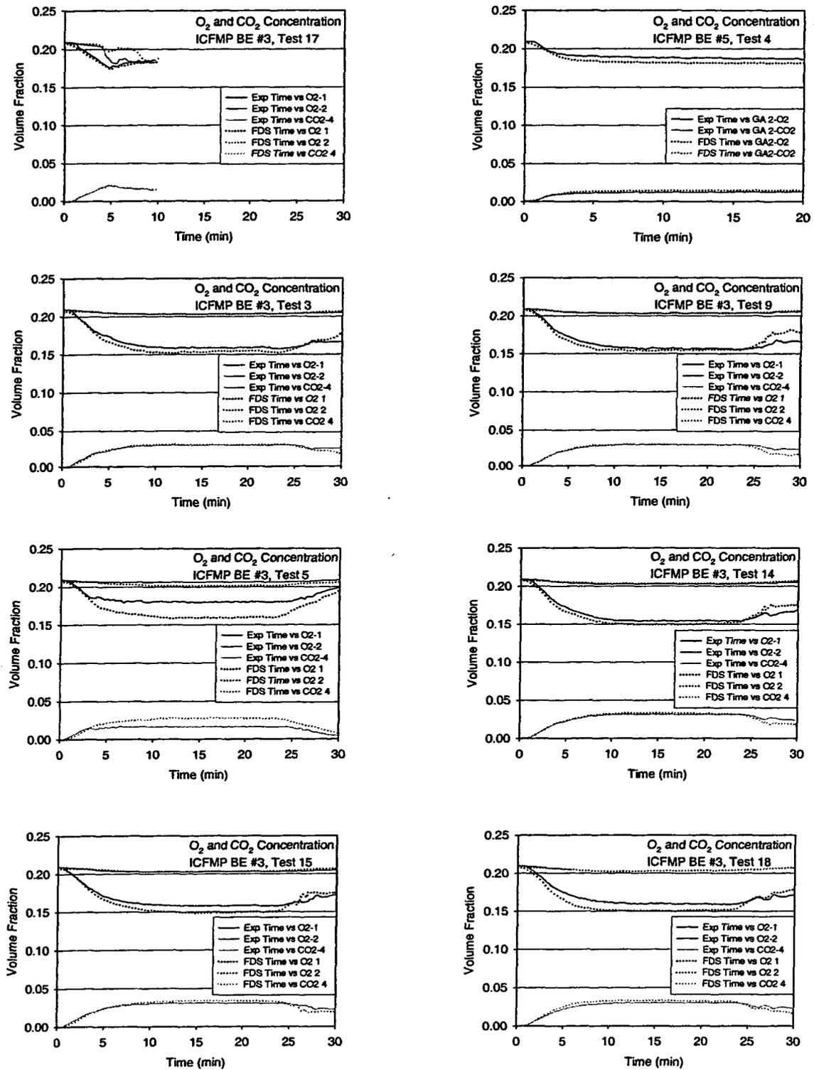
Figure A-27. O<sub>2</sub> and CO<sub>2</sub> concentration, ICFMP BE #3, open door tests. Note that the single test from ICFMP BE #5 is included at the upper right.
