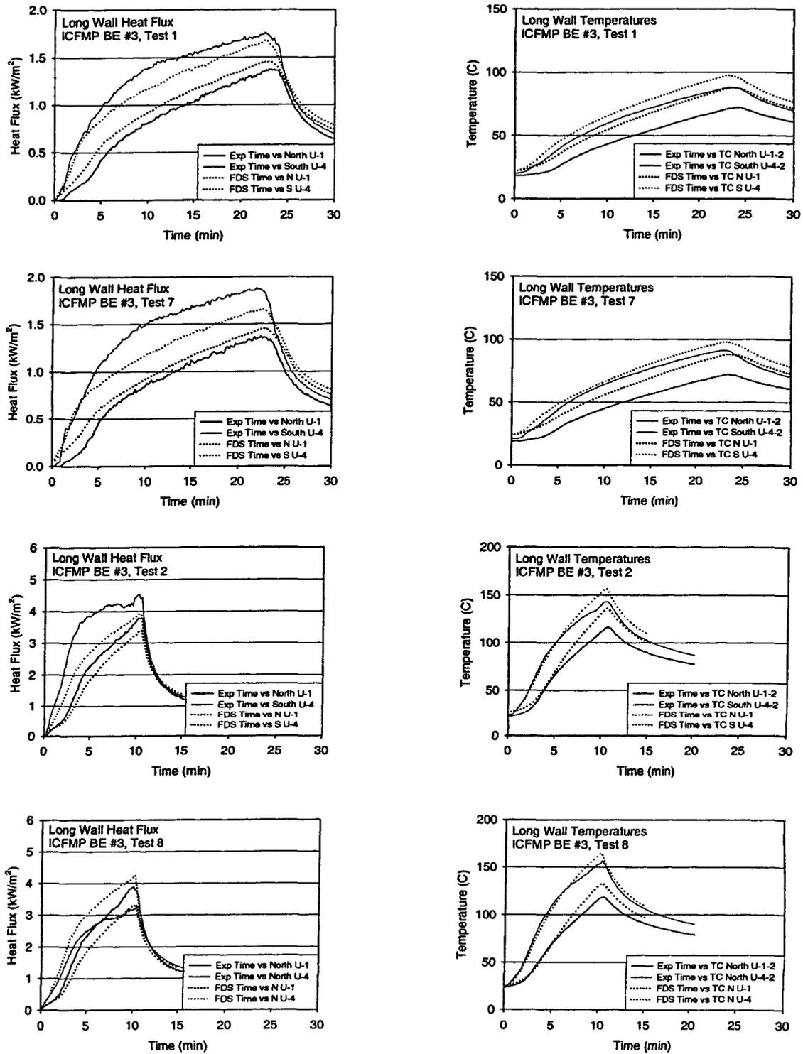
Figure A-65. Long wall heat flux and surface temperature, ICFMP BE #3, closed door tests.
