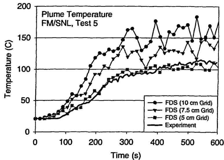
Figure 5-1. Grid sensitivity study for FM/SNL Test 5.
