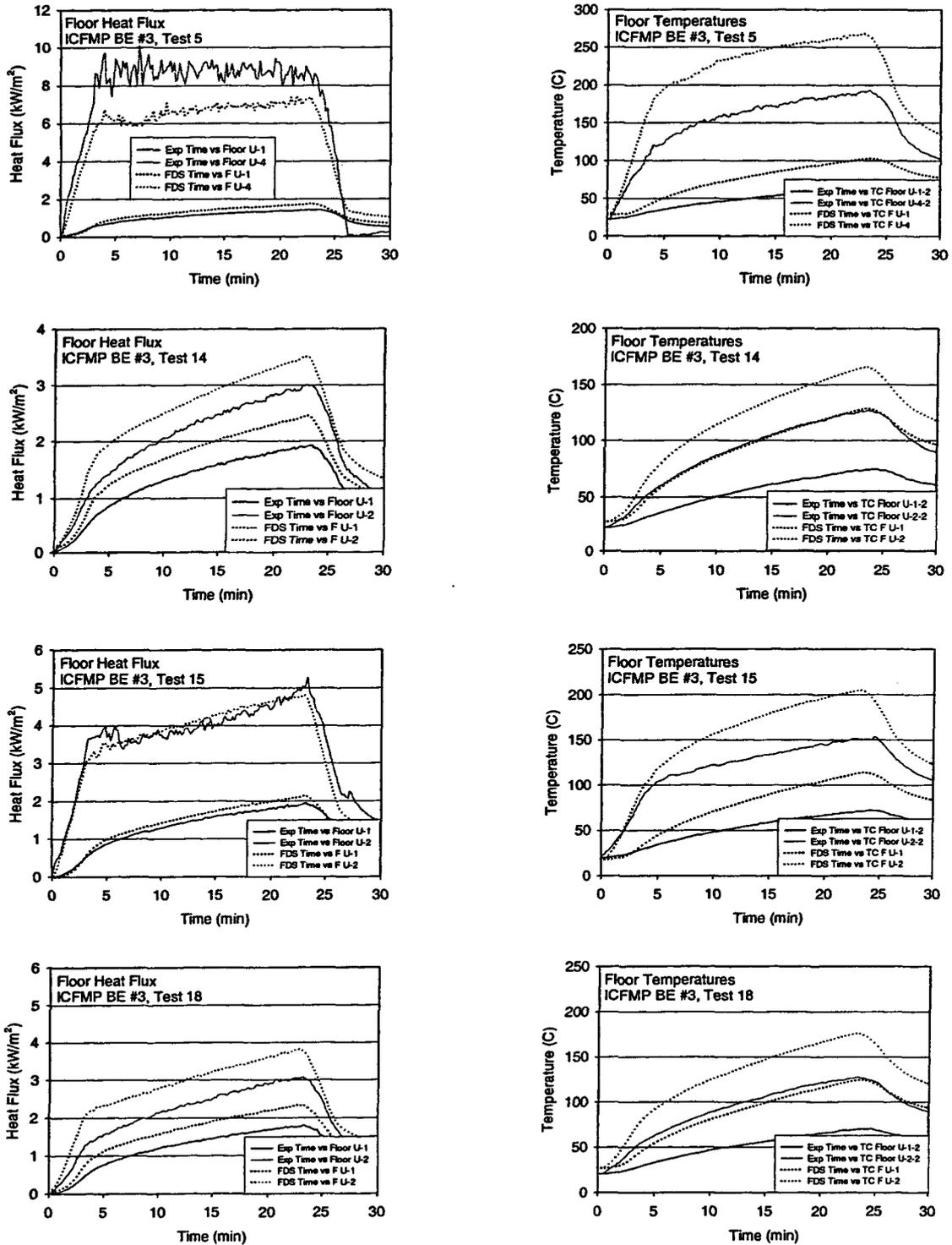
Figure A-80. Floor heat flux and surface temperature, ICFMP BE #3, open door tests.
