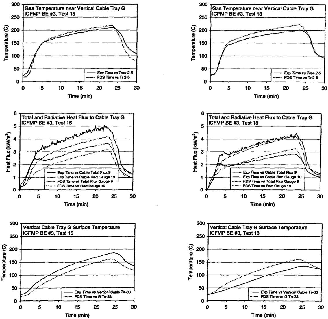
Figure A-59. Thermal environment near Vertical Cable Tray G, ICFMP BE #3, Tests 15 and 18.
