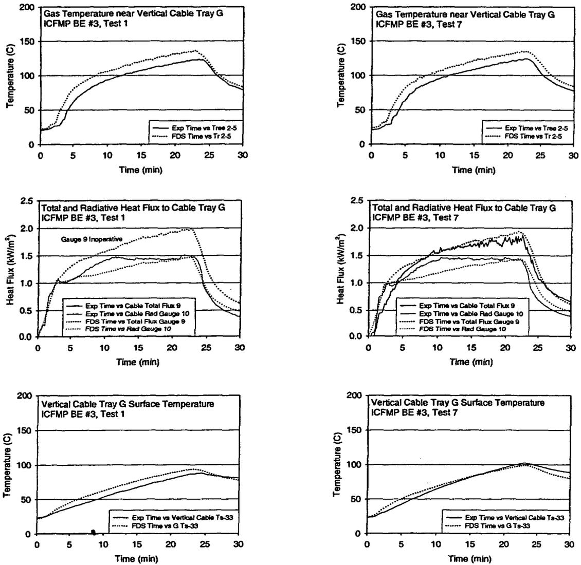
Figure A-53. Thermal environment near Vertical Cable Tray G, ICFMP BE #3, Tests 1 and 7.
