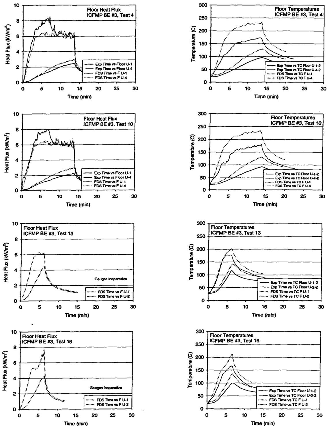
Figure A-78. Floor heat flux and surface temperature, ICFMP BE #3, closed door tests.
