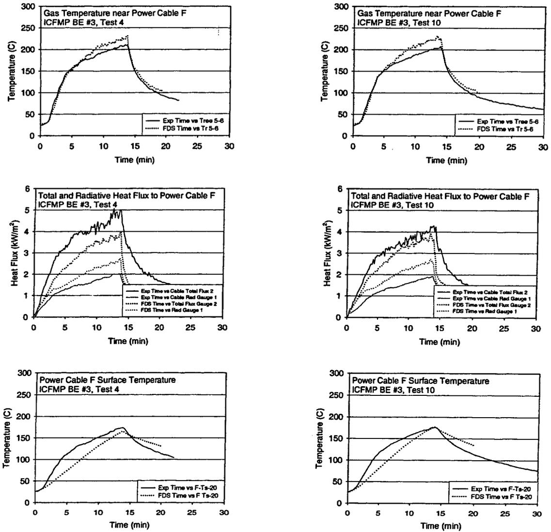
Figure A-48. Thermal environment near Power Cable F, ICFMP BE #3, Tests 4 and 10.
