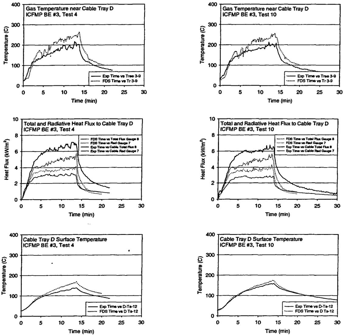
Figure A-41. Thermal environment near Cable Tray D, ICFMP BE #3, Tests 4 and 10.
