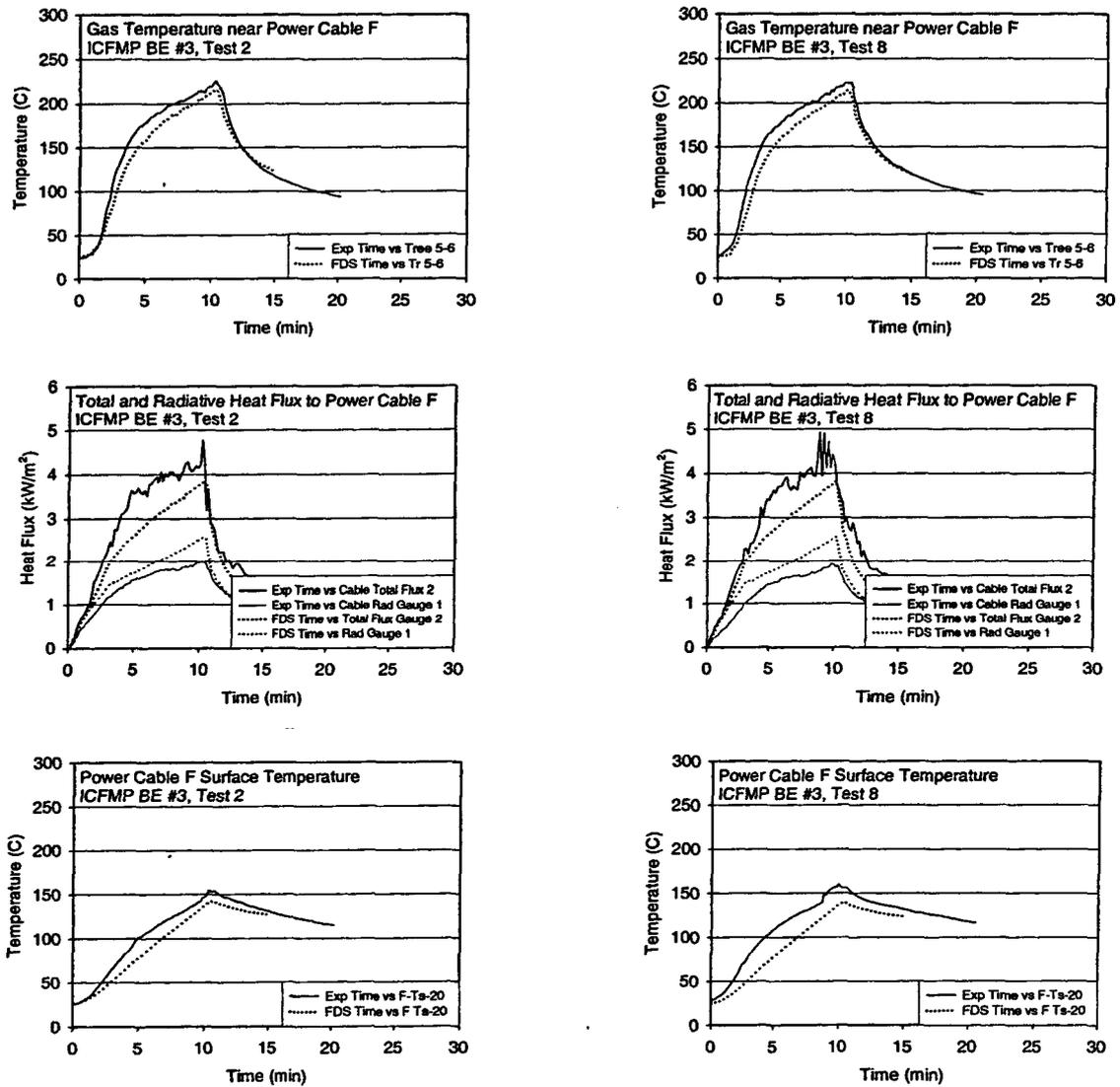
Figure A-47. Thermal environment near Power Cable F, ICFMP BE #3, Tests 2 and 8.
