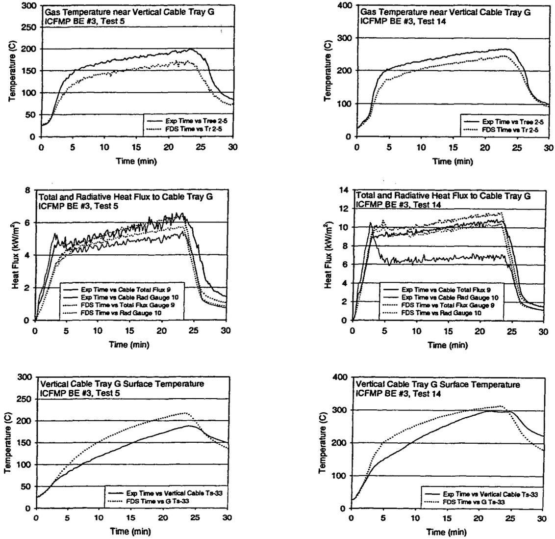
Figure A-58. Thermal environment near Vertical Cable Tray G, ICFMP BE #3, Tests 5 and 14.
