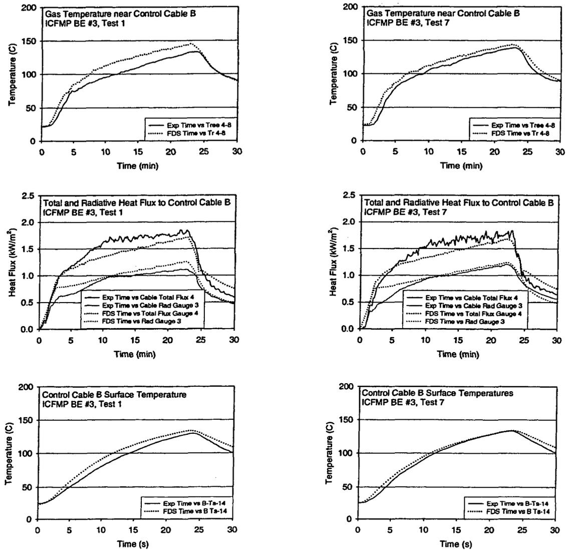
Figure A-32. Thermal environment near Cable B, ICFMP BE #3, Tests 1 and 7.
