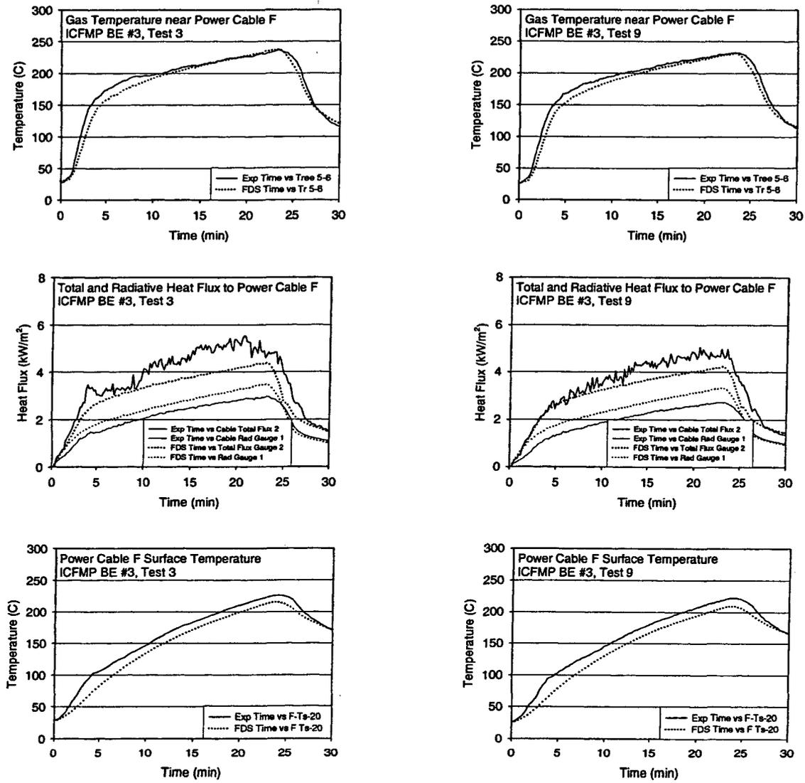
Figure A-50. Thermal environment near Power Cable F, ICFMP BE #3, Tests 3 and 9.
