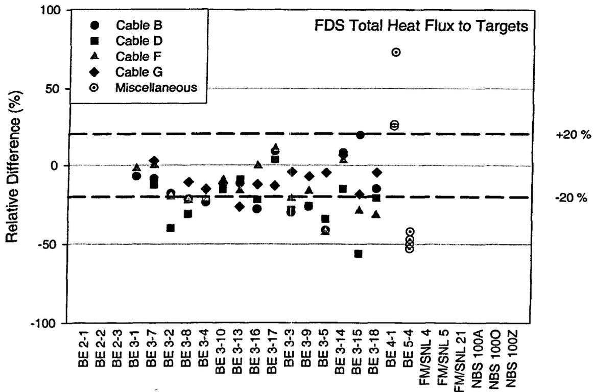
Figure 6-11. Summary of FDS predictions of heat flux to targets.
