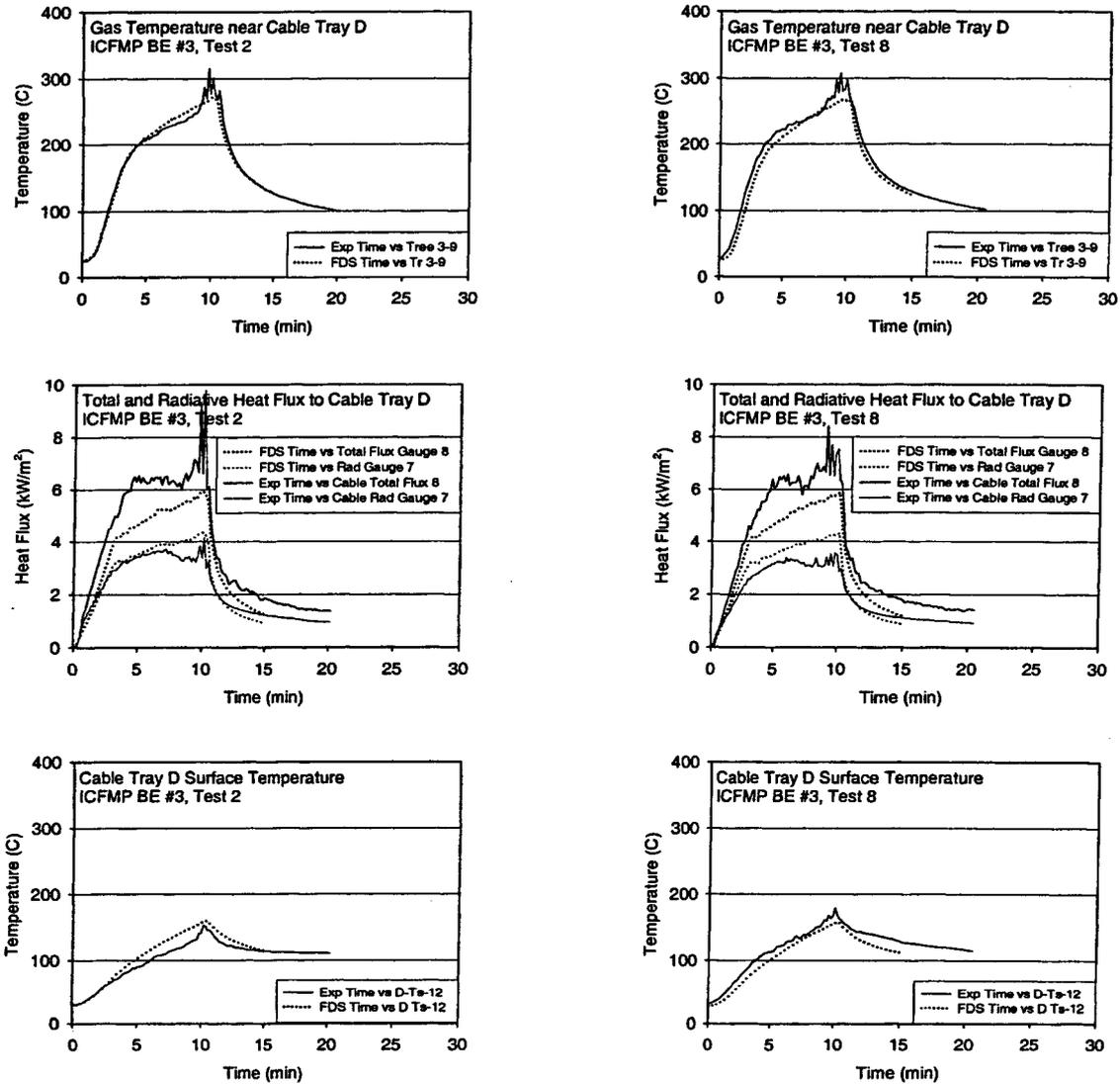
Figure A-40. Thermal environment near Cable Tray D, ICFMP BE #3, Tests 2 and 8.
