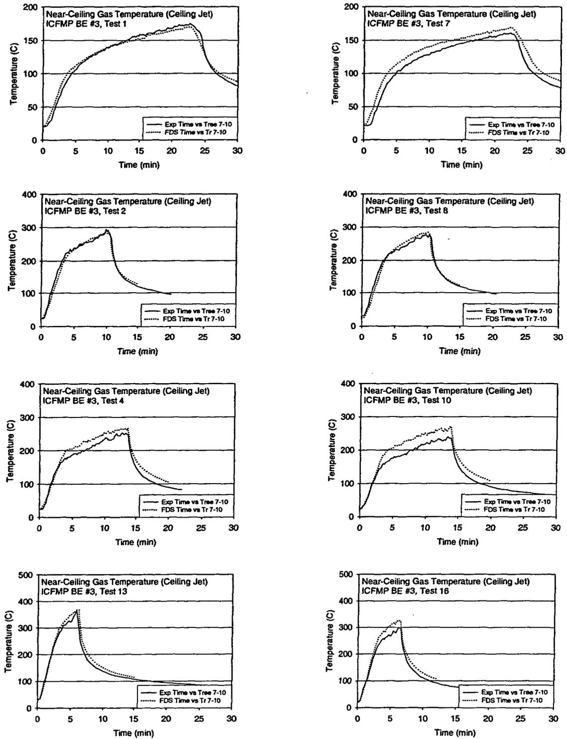
Figure A-18. Near-ceiling gas temperatures, ICFMP BE #3, closed door tests.
