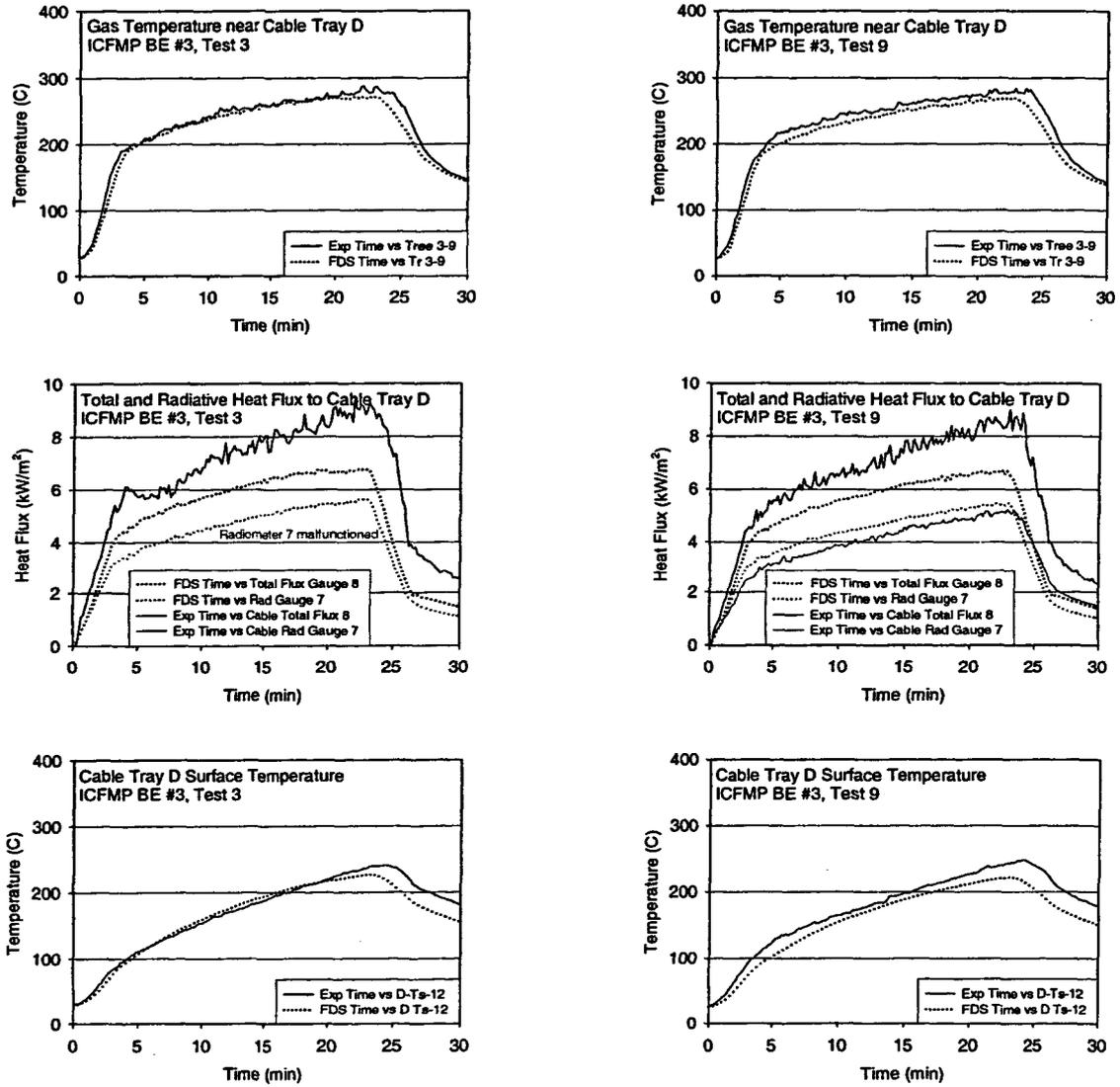
Figure A-43. Thermal environment near Cable Tray D, ICFMP BE #3, Tests 3 and 9.
