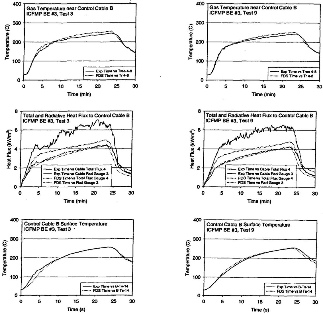
Figure A-36. Thermal environment near Cable B, ICFMP BE #3, Tests 3 and 9.
