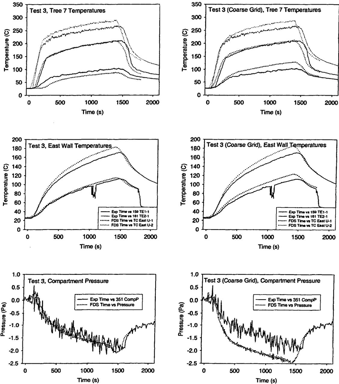
Figure 5-2. Fine (left) and coarse (right) simulations of ICFMP BE #3 Test 3.
