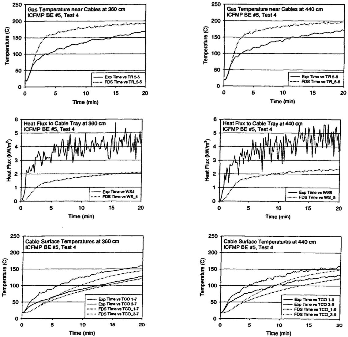
Figure A-64. Thermal environment near Vertical Cable Tray, ICFMP BE #5, Test 4.
