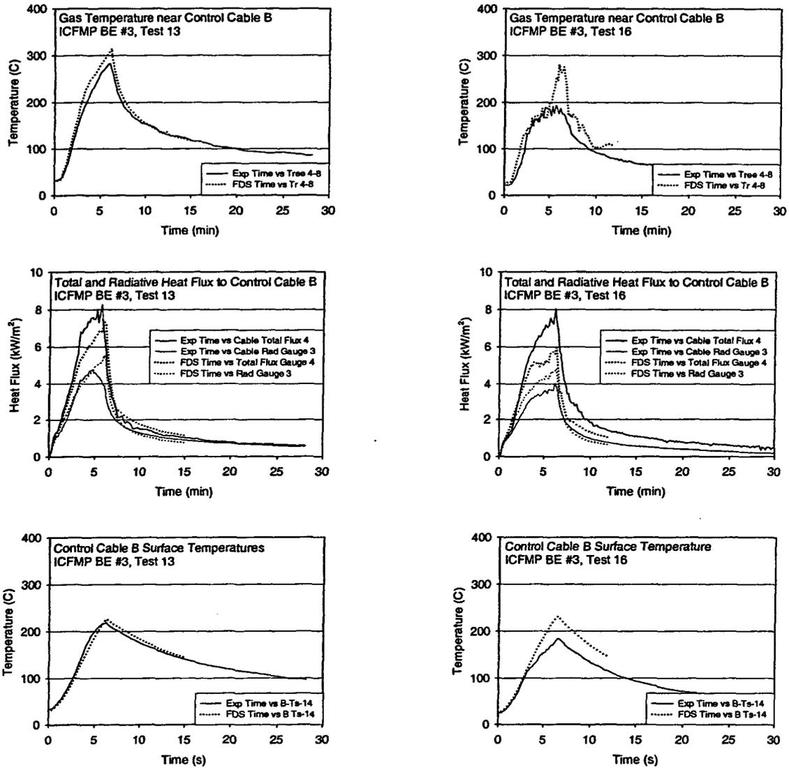
Figure A-35. Thermal environment near Cable B, ICFMP BE #3, Tests 13 and 16. Note the influence of the fan in Test 16.
