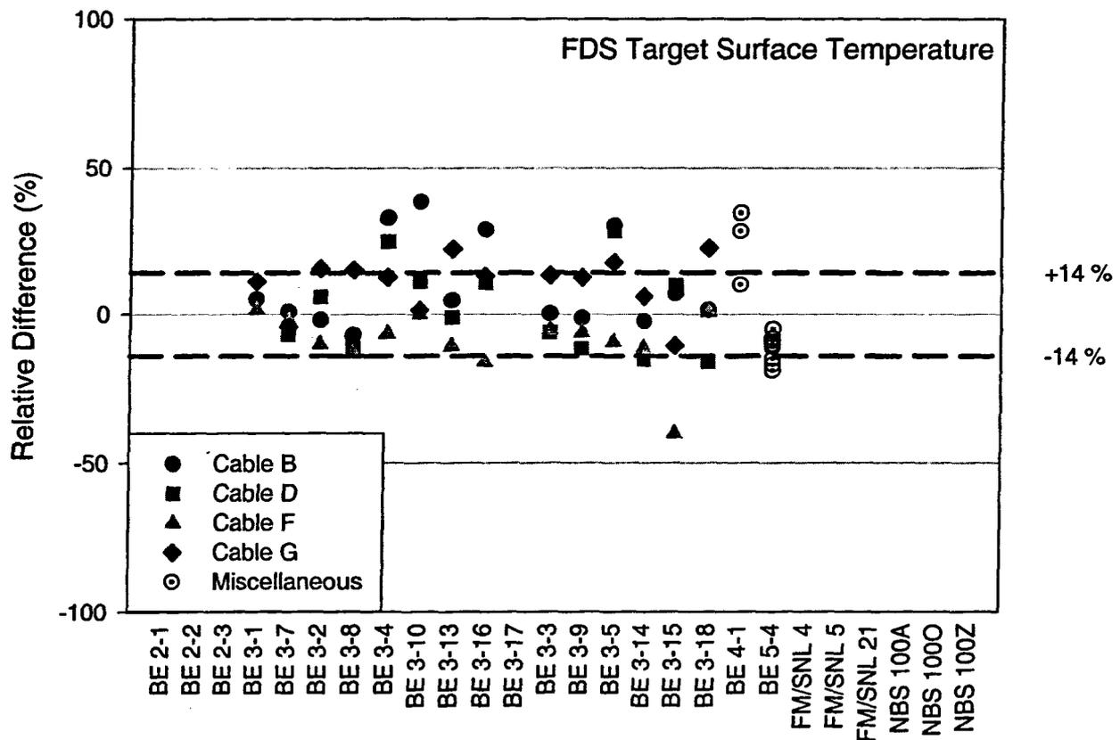
Figure 6-10. Summary of FDS predictions of target temperature.
