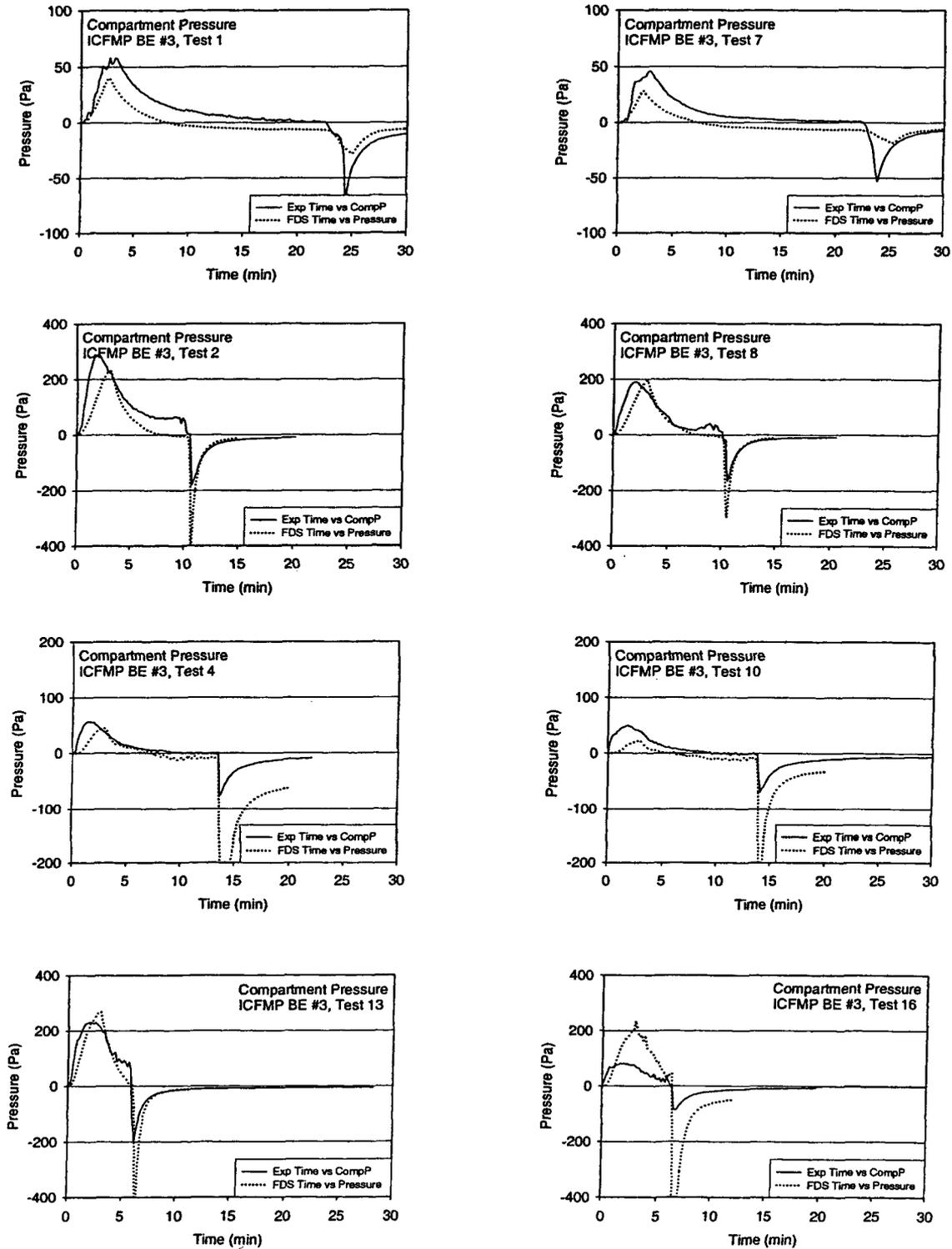
Figure A-30. Compartment pressure, ICFMP BE #3, closed door tests.
