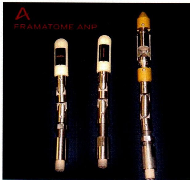
Figure 5: UT probes for BMI examination included circumferential, axial & 0° configurations
