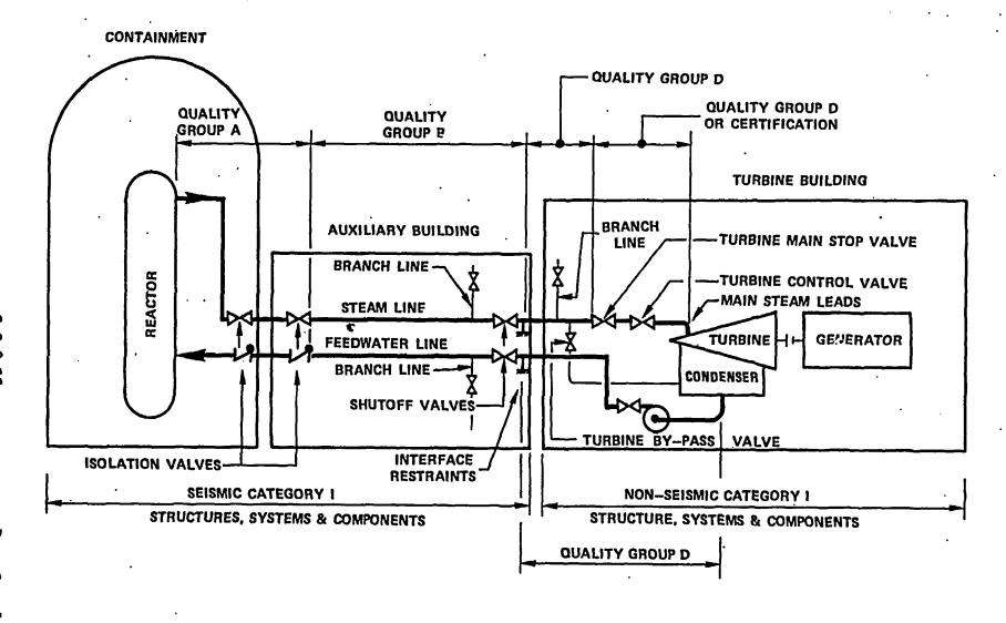
Figure B-1 NRC Quality Group and Seismic Category Classifications Applicable to Power Conversion System Components in BWR/6 Plants.
