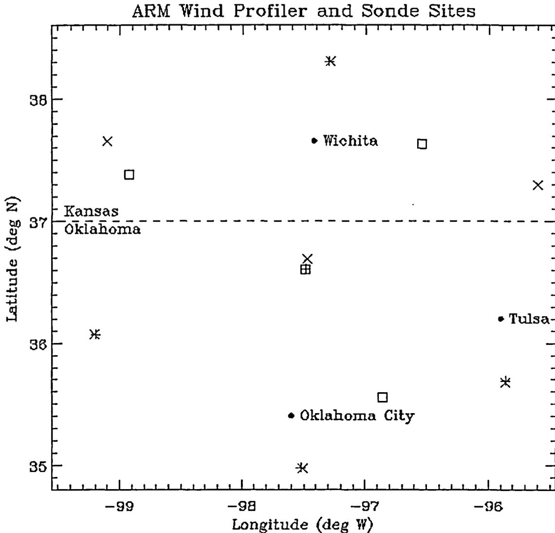
**Figure 2.** Location of ARM Upper Air Observations. + indicates sonde and AERI sites, x indicates NOAA Profiler sites, and □ 915 MHz RWP/RASS sites. Note that some sites have multiple measurements, and the Central Facility has all three types.
