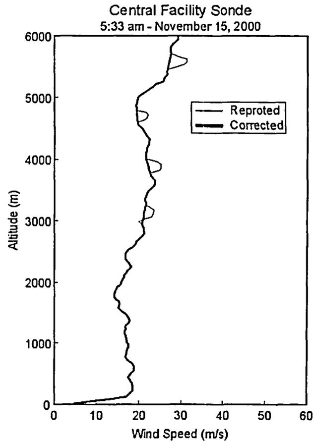
**Figure 7.** Central Facility Sonde Launched at 5:33 am CST on November 15, 2000. Quite a few of the sondes exhibited speed anomalies in an otherwise fairly smooth profile. They were often associated with a missing layer in the data. They were corrected by interpolating between the bottom and top of the anomaly. Note that direction was hardly affected.
