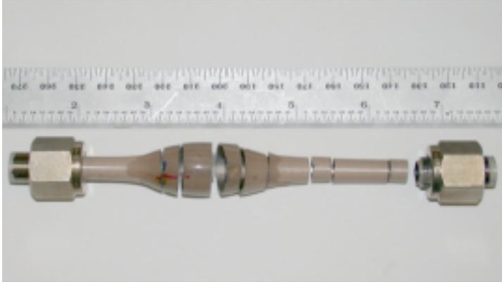
Figure 3.26. Steam-preoxidized Zircaloy-4 specimen after air oxidation with internal Ar pressure of 400 psi in Test 4.
