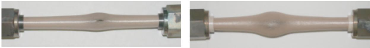
Figure 3.31. Zircaloy-4 specimens tested with internal pressure of (left) 400 and (right) 200 psig at 700°C.
