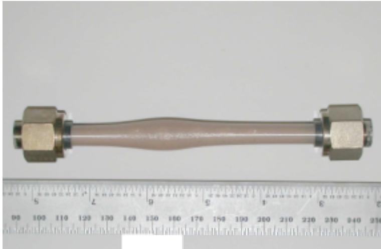
Figure 3.29. Steam-preoxidized Zircaloy-4 specimen with internal Ar pressure of 400 psi after oxidation in air for 47 h (end of test) in Test 5.
