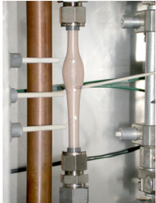
*Figure 3.25. Steam-preoxidized Zircaloy-4 specimen with an internal Ar pressure of 400 psi after 22 h elapsed time and at the end of Test 4 at  $\approx 40$  h.*
