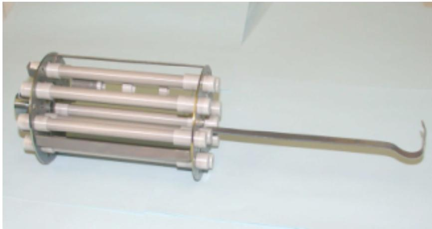
*Figure 2.7. 150-mm-long specimens of Zircaloy-4 specimens after oxidation in steam for 140 h at 550°C.*
