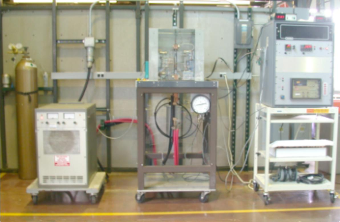
*Figure 2.9. Experimental setup for air oxidation studies on Zircaloy cladding tubes with internal pressure.*
