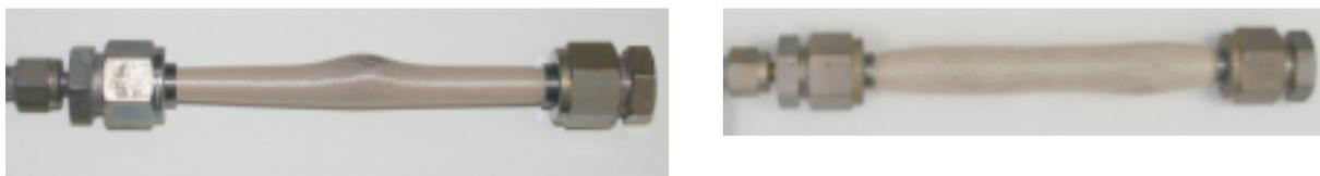
Figure 3.32. Zircaloy-4 specimens tested with internal pressure of (left) 175 and (right) 100 psig at 800°C.
