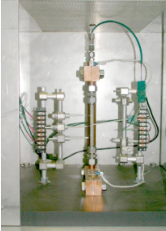
*Figure 3.24. Steam-preoxidized Zircaloy-4 specimen setup with an internal Ar pressure of 400 psi in Test 4.*
