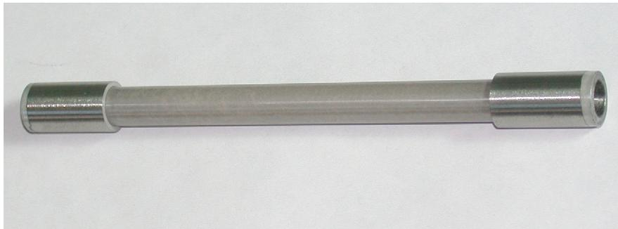
*Figure 2.8. Zircaloy-4 specimen after steam oxidation, sleeve grinding, and end drilling. This specimen is ready for air oxidation test under internal pressure.*
