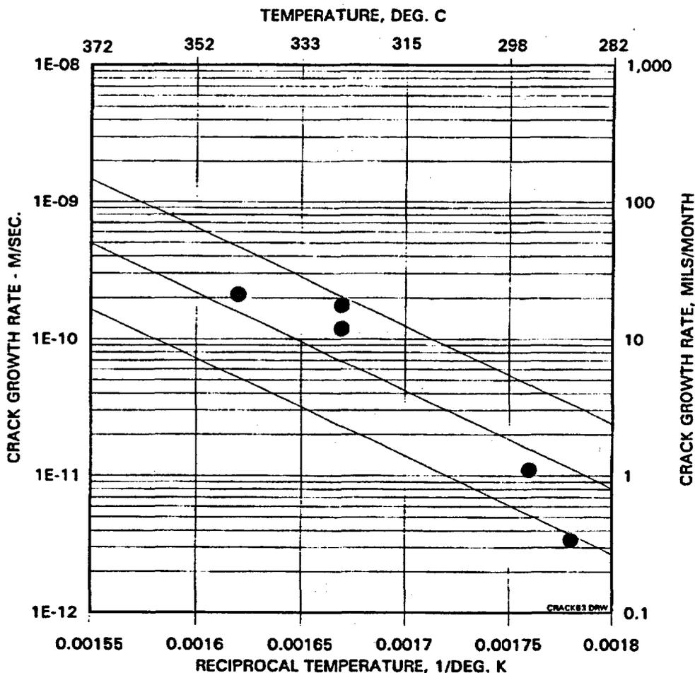
Figure 4-7 Effects of Temperature on Growth Rates: Alloy 182 [3]
