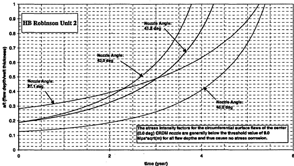
Figure 4-4 Crack Growth Prediction for Circ Outside Surface Flaws Along the Top of the Weld
