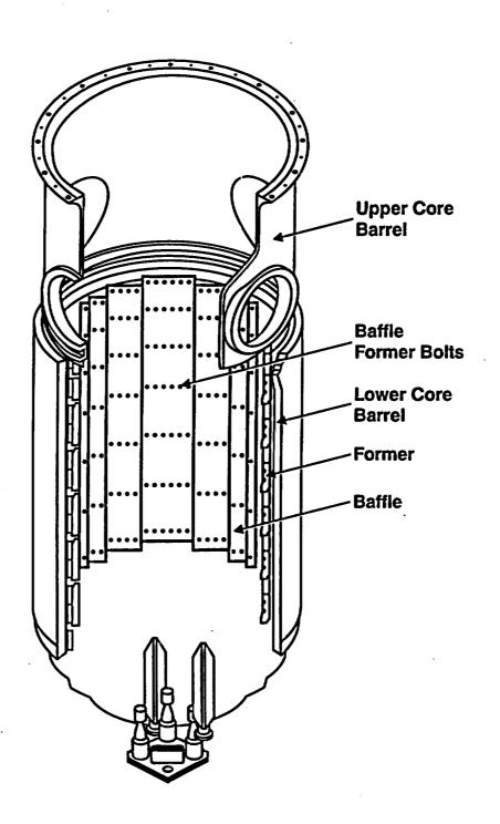
Typical PWR Reactor Vessel Internals
