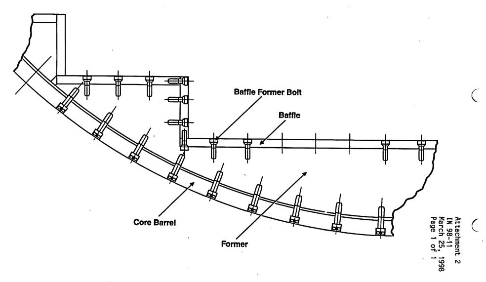
Typical PWR Core Barrel, Former, and Baffle Arrangement
