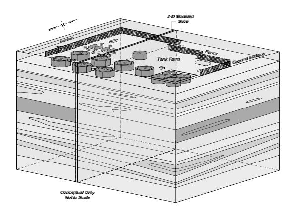
Figure 4. Illustration of the two-dimensional modeling slice used in PORFLOW
