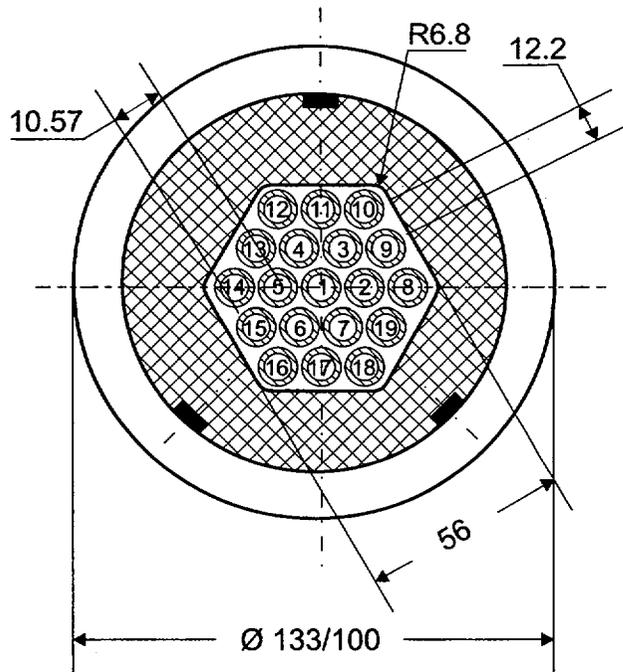
Figure 2: Cross section of the core
