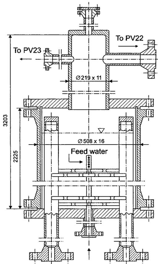
Figure 3: The SG model of the PMK-2 facility
