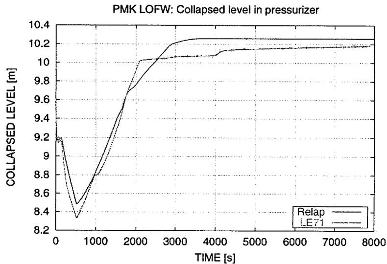
Figure 12: Collapsed level in the PRZ
