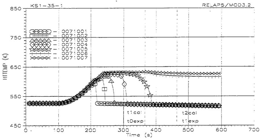
Fig. B-4. RELAP5/MOD3.2-calculated TW(t) heated tube inside wall temperatures histories in the upper, middle and bottom parts of the FA model (tcal=0-600 s).
