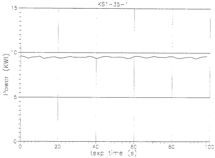
Fig. A-1. FA model heat release power history  $W(t)$  ( $t_{exp}=0-100$  s).
