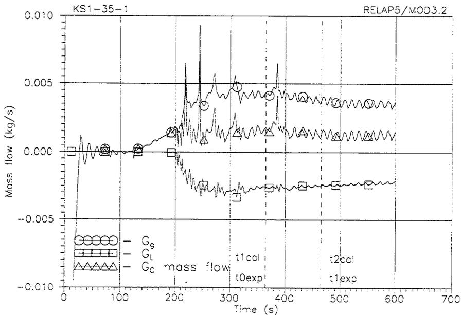
Fig. 4.5. RELAP5/MOD3.2- calculated  $G_{g1}(t)$  mass flow rate of generated steam and  $G_{L1}(t)$  steam condensate mass flow rate histories under CCF conditions at Core Model outlet ( $t_{cal}=0-600$  s), and also selection of time interval, corresponding  $D_{texp}$ , and selection of time moment  $t_{1cal}$ , corresponding  $t_{0exp}$  for KS-1 Test.
