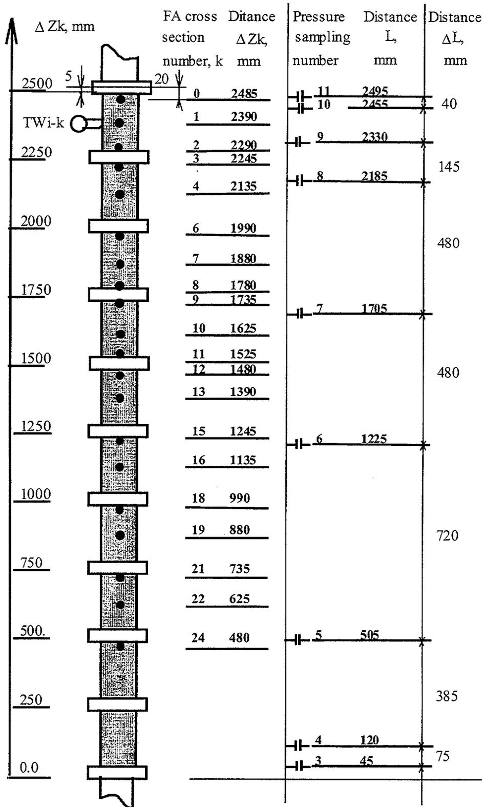
Fig. 2.5. Scheme of location of the thermocouples  $TW_{i-k}$  and pressure sampling points along the FA model height.
