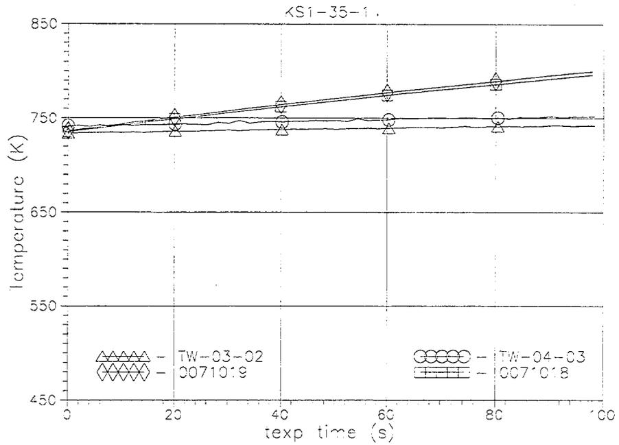
Fig. B-16. Comparison of measured TW03-02(t), TW04-03(t) and RELAP5/MOD3.2-calculated heated tube inside wall temperatures histories in the upper part of FA model (texp=0-100 s).
