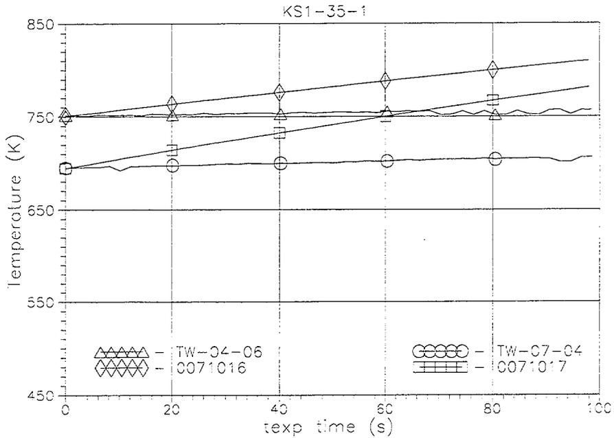
Fig. C-6. Comparison of measured TW07-04(t), TW04-06(t) and RELAP5/MOD3.2-calculated heated tube inside wall temperatures histories in the upper part of FA model (texp=0-100 s)
