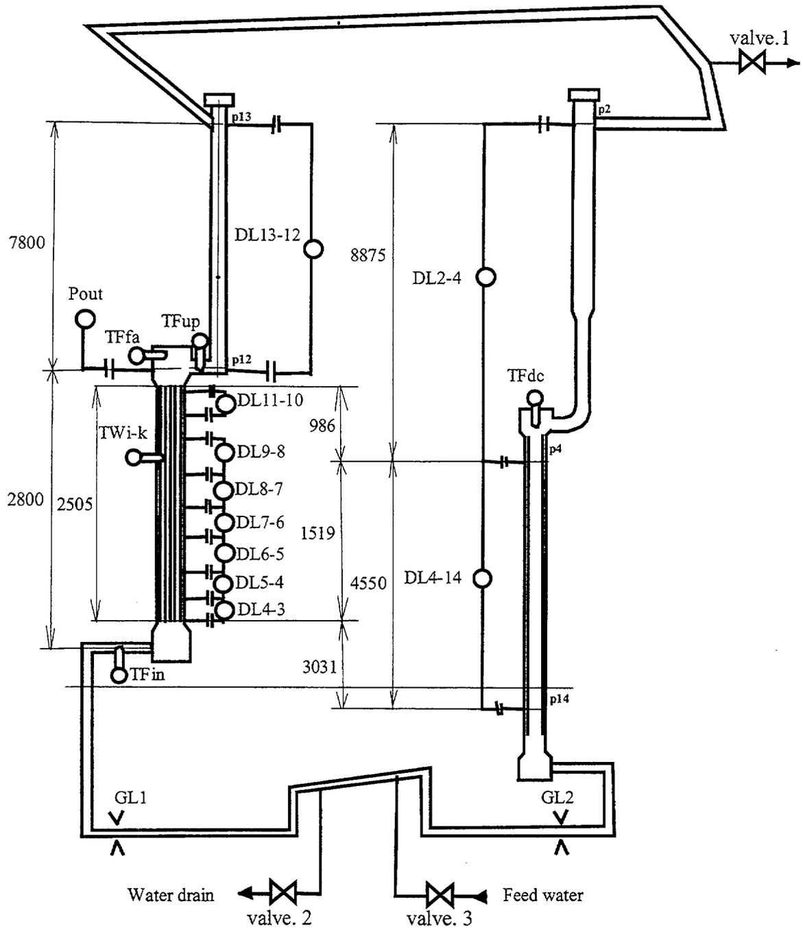
Fig. 2.4. Measurements scheme in the VVER primary system model.
