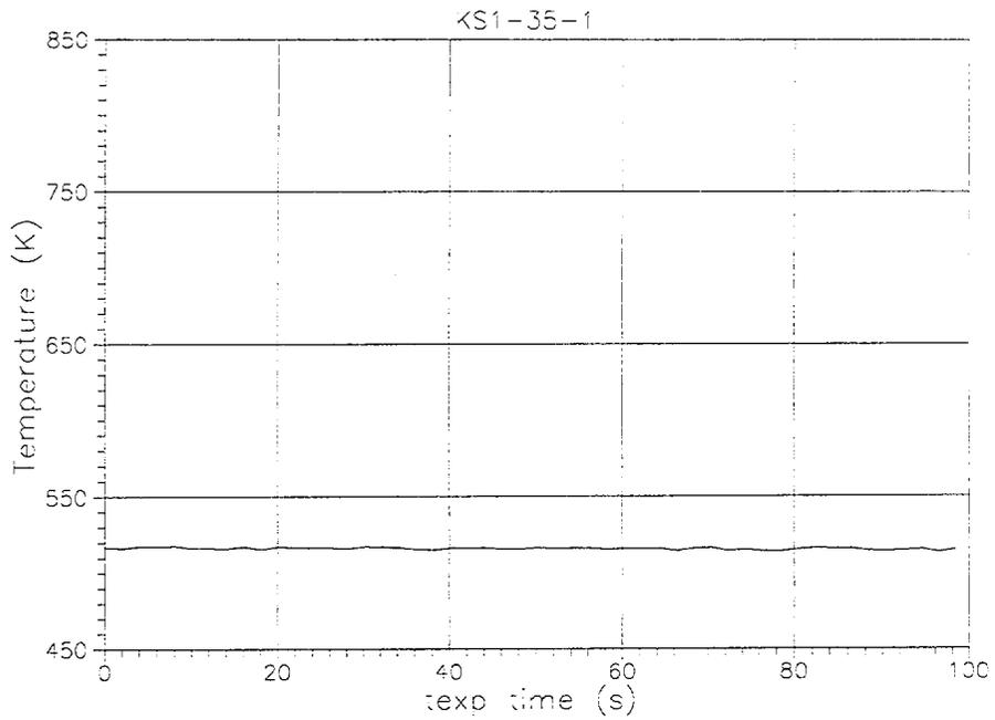
Fig. A-3. Measured  $T_{Fin}(t)$  Core model inlet coolant temperature history ( $t_{exp}=0-100$  s).
