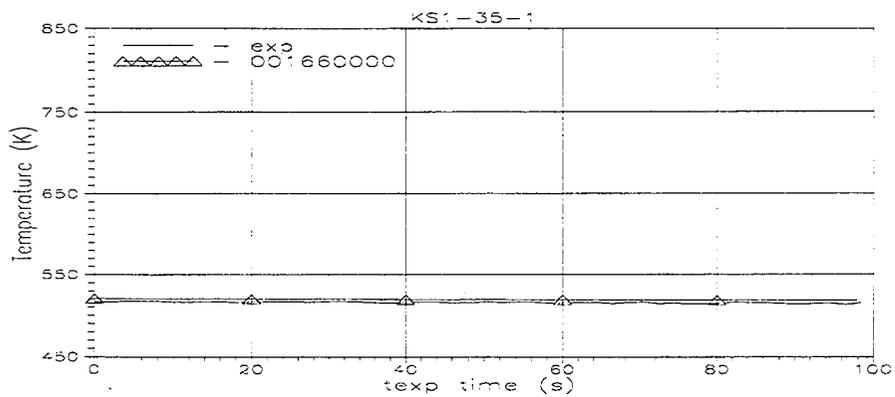
Fig. B-3. Comparison of measured and RELAP5/MOD3.2-calculated  $T_{Fin}(t)$  coolant temperature at Core model inlet ( $t_{exp}=0-100$  s).
