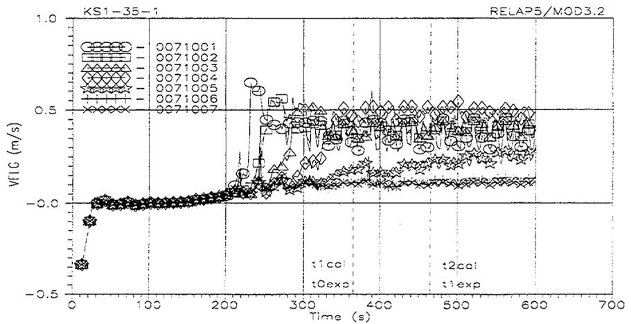
Fig. B-8. RELAP5/MOD3.2-calculated  $V_g(t)$  junction vapor velocities histories in the upper, middle and bottom parts of FA channel ( $t_{cal}=0-600$  s).
