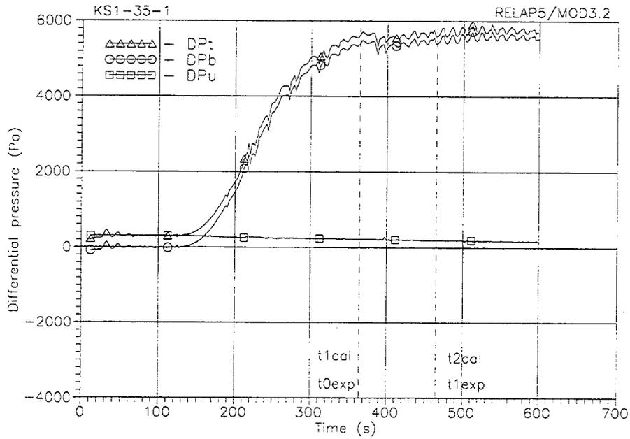
Fig. 4.4. RELAP5/MOD3.2-calculated  $D_{pt}(t)$  Core Model total differential pressure,  $D_{pu}(t)$ , core upper half part differential pressure and  $D_{pb}(t)$  core bottom half part differential pressure histories, and also selection of time interval, corresponding  $D_{texp}$ , and selection of time moment  $t_{1cal}$ , corresponding  $t_{0exp}$  for KS-1 Test ( $t_{cal}=0-600$  s).
