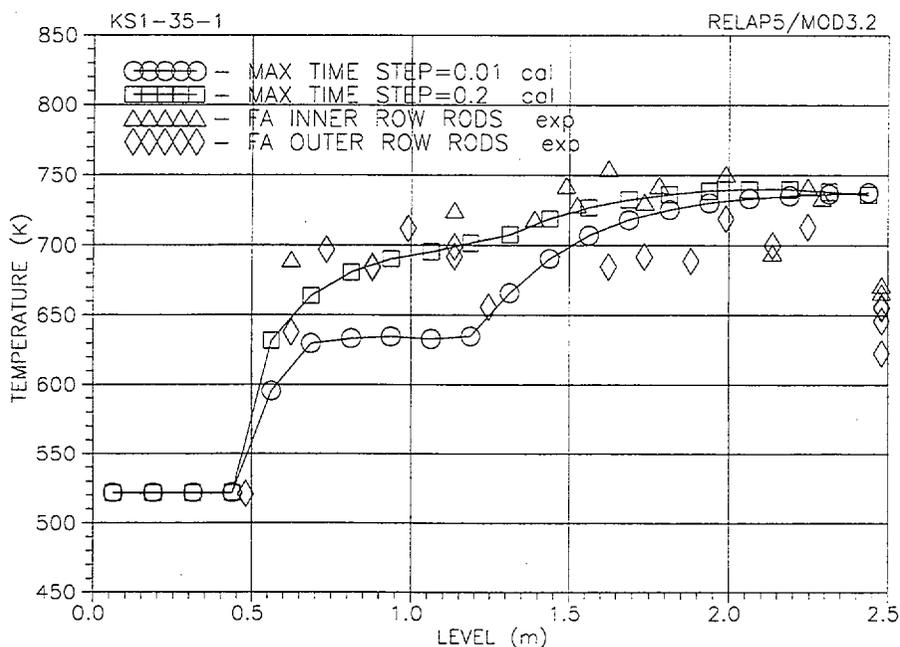
Fig. 5.1. Comparison of RELAP5/MOD3.2-calculated core axial inside wall temperatures profile in the bundle heated tube for time moment  $t_{cal}=365$  s, corresponding  $t_{0exp}$  for KS-1 Test, and experimental core axial distribution of temperatures of rod simulators  $T_{Wi-k}$  of the FA Model for time moment  $t_{0exp}$ .
