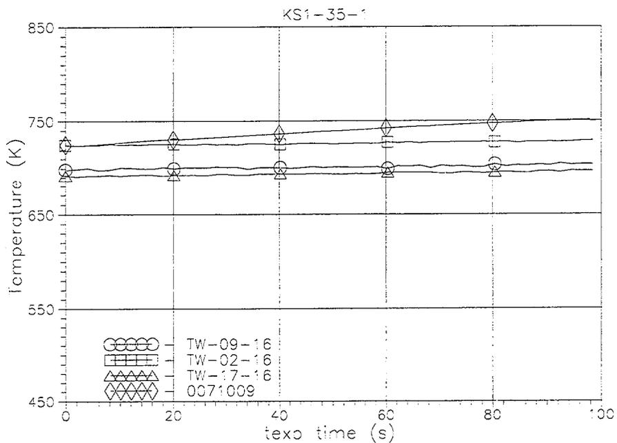
Fig. C-10. Comparison of measured TW09-16(t), TW02-16(t), TW17-16(t) and RELAP5/MOD3.2-calculated heated tube inside wall temperatures histories in the middle part of FA model (texp=0-100 s)
