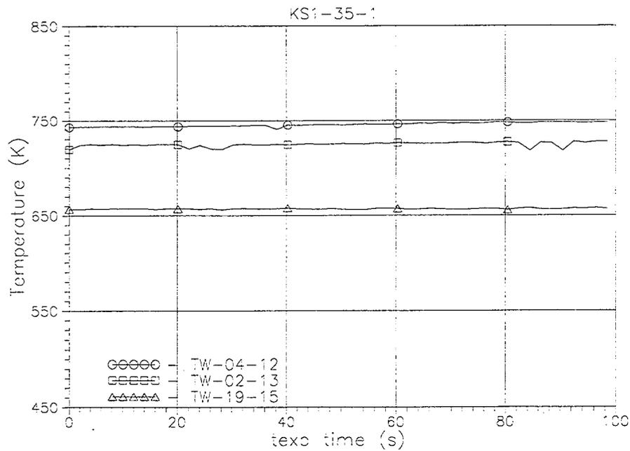
Fig. A-12. Measured TW04-12(t), TW02-13(t) and TW19-15(t) heated tube inside wall temperatures histories in the middle part of the FA model (texp=0-100 s).
