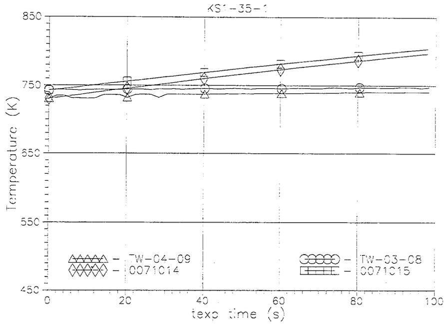
Fig. C-7. Comparison of measured TW03-08(t), TW04-09(t) and RELAP5/MOD3.2-calculated heated tube inside wall temperatures histories in the upper part of FA model (texp=0-100 s)
