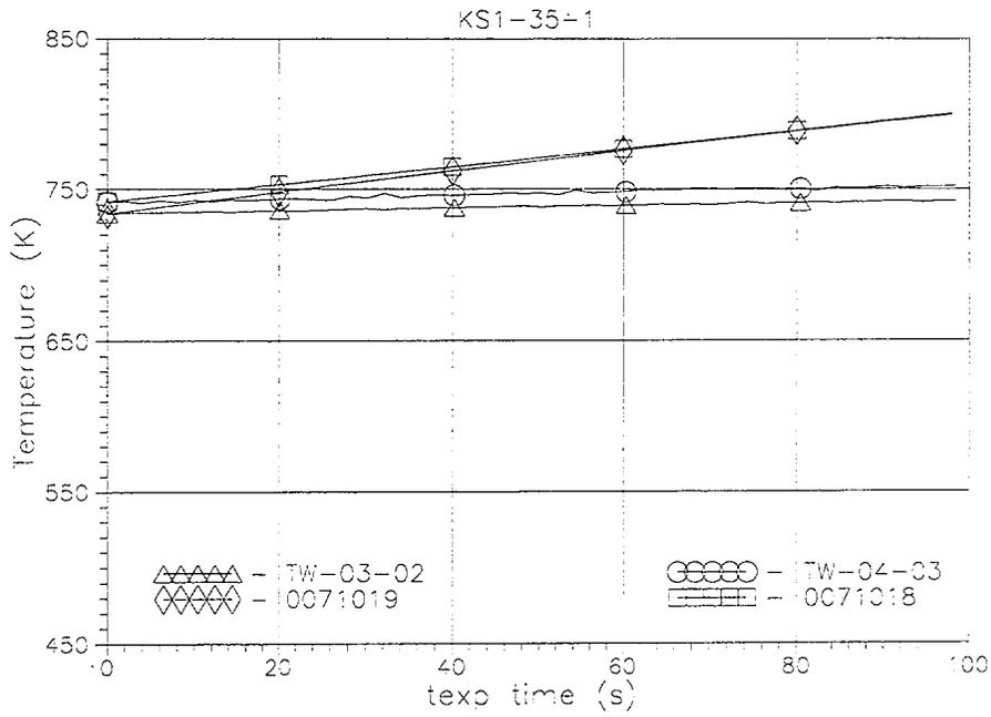
Fig. C-5. Comparison of measured TW03-02(t), TW04-03(t) and RELAP5/MOD3.2-calculated heated tube inside wall temperatures histories in the upper part of FA model (texp=0-100 s)
