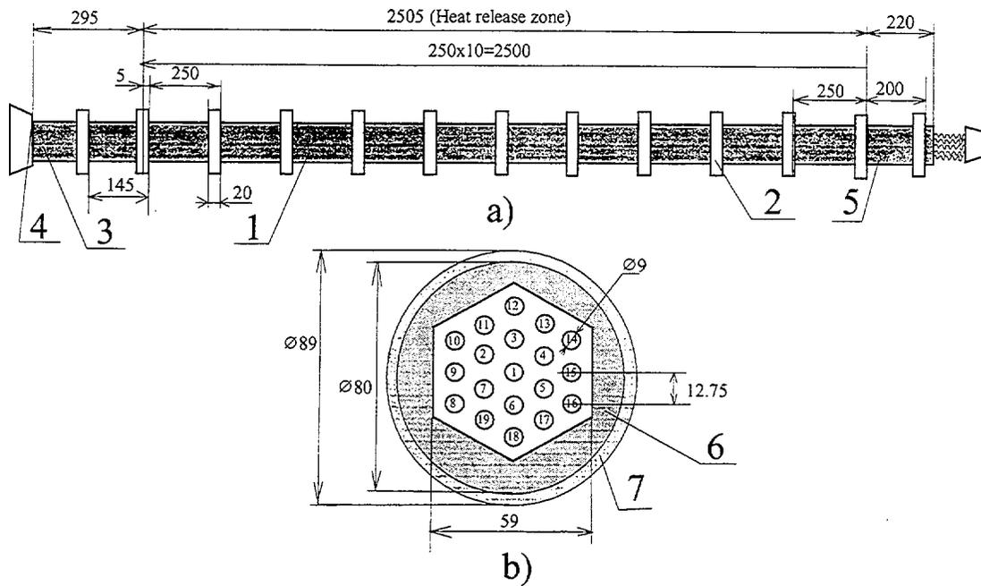
Fig.2.3. Model of the VVER-1000 fuel assembly.
