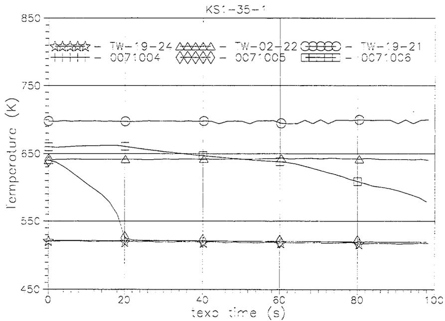
Fig. C-12. Comparison of measured TW19-21(t), TW02-22(t), TW19-24(t) and RELAP5/MOD3.2-calculated heated tube inside wall temperatures histories in the bottom part of FA model (texp=0-100 s)
