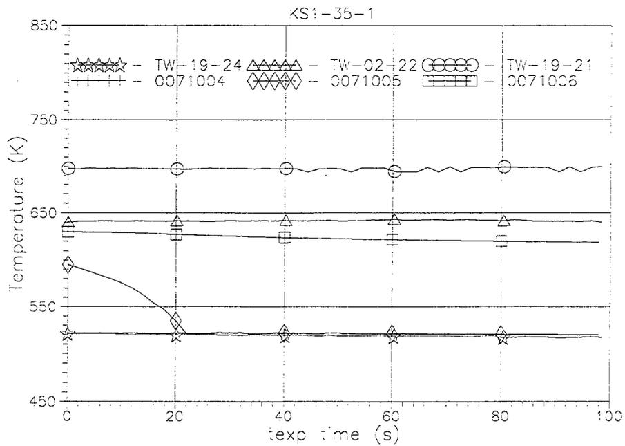
Fig. B-23. Comparison of measured TW19-21(t), TW02-22(t), TW19-24(t) and RELAP5/MOD3.2-calculated heated tube inside wall temperatures histories in the bottom part of FA model (texp=0-100 s).
