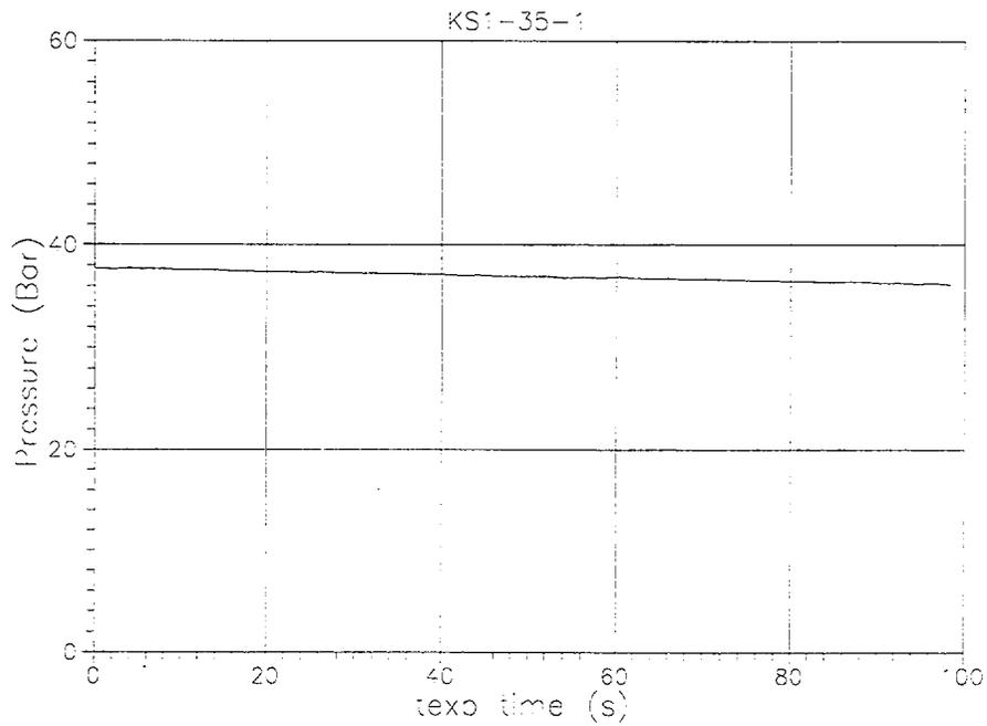
Fig. A-2. Measured  $P_{out}(t)$  Core model outlet pressure history ( $t_{exp}=0-100$  s).
