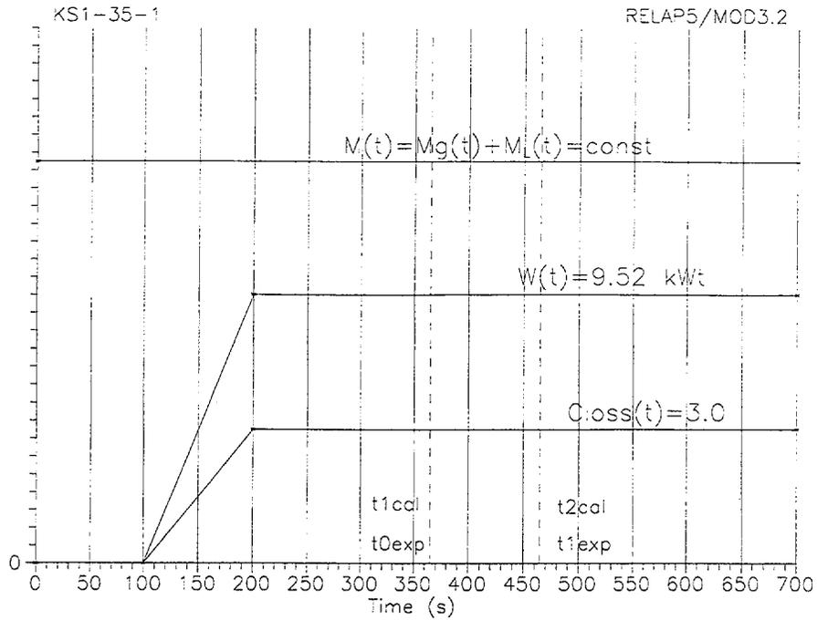
Fig. 4.2. Variation of FA Model power  $W(t)$ , correctional coefficient of heat losses  $C_{loss}(t)$  and coolant mass inventory  $M=M_L+M_G$  in the closed loop during calculation procedures for modeling of KS-1 Test ( $t_{cal}=0-600$  s).
