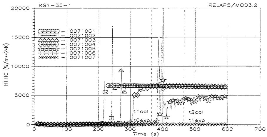
Fig. B-6. Behavior of RELAP5/MOD3.2-calculated  $H_{w1}(t)$  coefficient of heat transfer from outer surfaces of rod simulators to coolant in the upper, middle and bottom parts of FA model ( $t_{cal}=0-600$  s).
