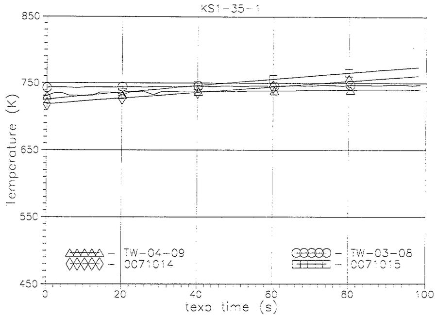
Fig. B-18. Comparison of measured TW03-08(t), TW04-09 (t) and RELAP5/MOD3.2-calculated heated tube inside wall temperatures histories in the upper part of FA model (texp=0-100 s).
