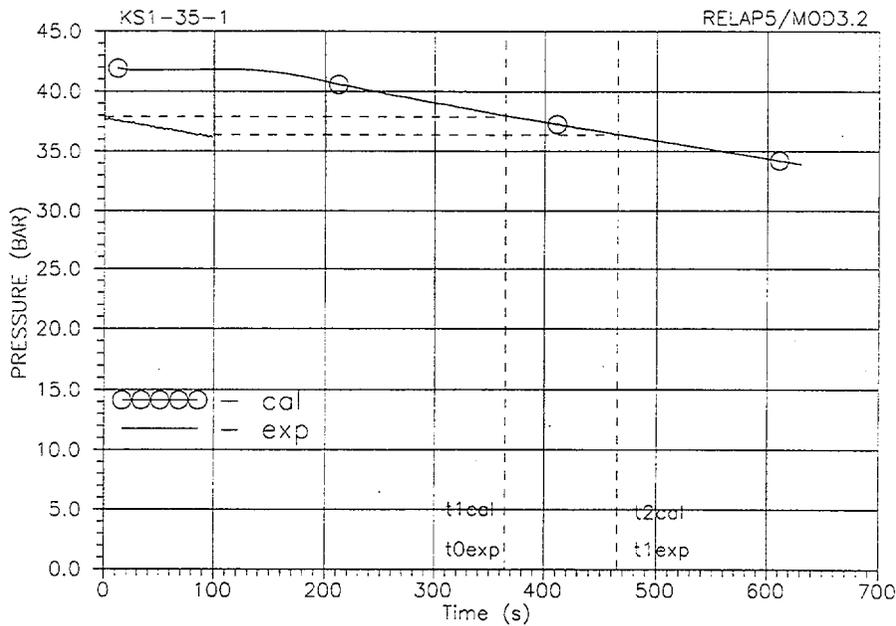
Fig. 4.3. Comparison of RELAP5/MOD3.2-calculated  $P_{out}(t)_{cal}$  ( $t_{cal}=0-700$  s) and experimental  $P_{out}(t)_{exp}$  curves of pressure decrease, and also selection of time interval, corresponding  $\Delta t_{exp}$ , and selection of time moment  $t_{1cal}$ , corresponding  $t_{0exp}$  for KS-1 Test.
