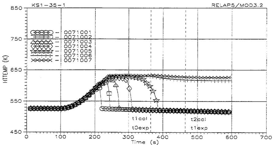
Fig. 4.6. RELAP5/MOD3.2-calculated TW(t) heated tube inside wall temperatures histories in the upper, middle and bottom parts of the FA Model ( $t_{cal}=0-600$  s), and also selection of time interval, corresponding  $D_{exp}$ , and selection of time moment  $t1_{cal}$ , corresponding  $t0_{exp}$  for KS-1 Test.
