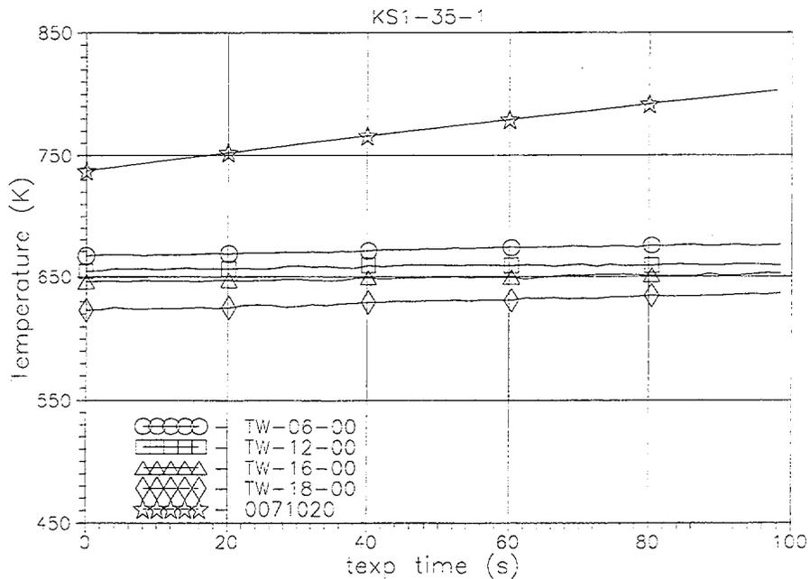
Fig. B-15. Comparison of measured TW06-00(t), TW12-00(t), TW16-00(t), TW18-00(t) and RELAP5/MOD3.2-calculated heated tube inside wall temperatures histories at the top of FA model (texp=0-100 s).
