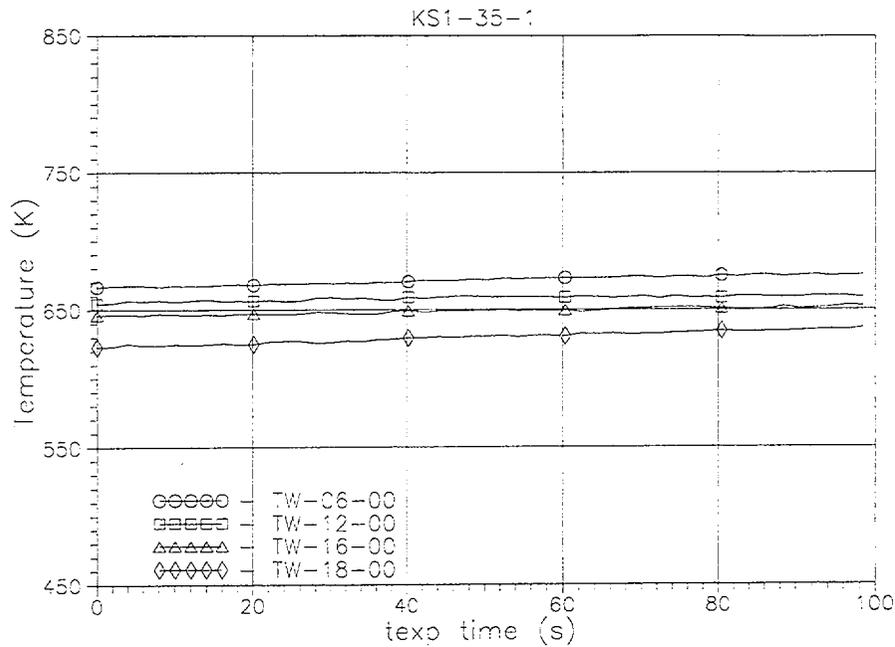
Fig. A-7. Measured TW06-00(t), TW12-00(t), TW16-00(t) and TW18-00(t) heated tube inside wall temperatures histories at the top of the FA model (texp=0-100 s).
