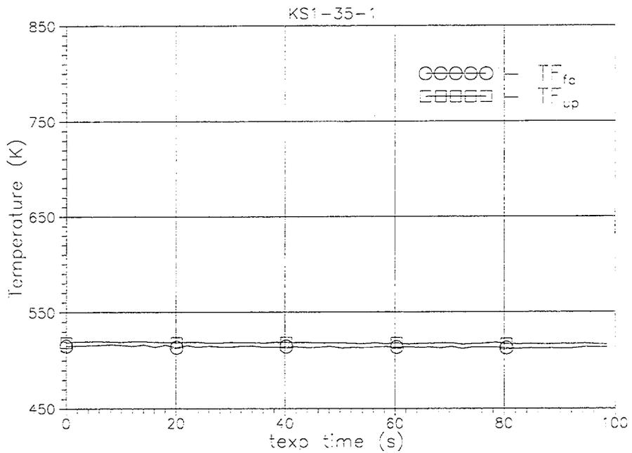
Fig. A-4. Measured  $T_{fa}(t)$  FA model outlet and  $T_{up}(t)$  UP model inlet coolant temperatures histories ( $t_{exp}=0-100$  s).
