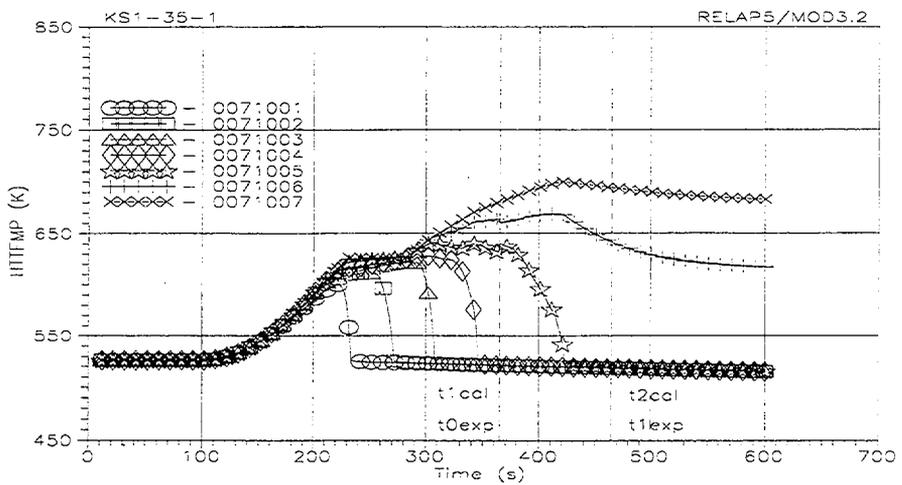
Fig. C-2. RELAP5/MOD3.2-calculated TW(t) heated tube inside wall temperatures histories in the upper, middle and bottom parts of the FA model (tcal=0-600 s). Maximum time step =0.2 s. Restart time t=365 s.
