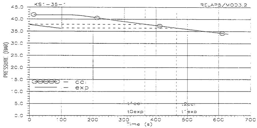
Fig. B-1. RELAP5/MOD3.2-calculated  $P_{out}(t)_{cal}$  pressure at Core model outlet ( $t_{cal}=0-600$  s).
