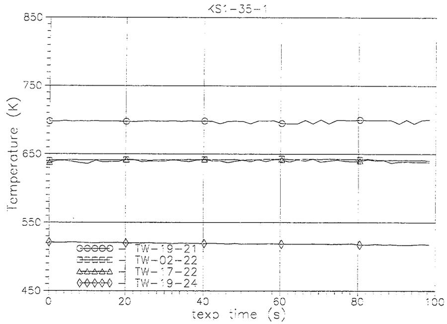
Fig. A-15. Measured TW19-21(t), TW02-22(t), TW17-22(t) and TW19-24(t) heated tube inside wall temperatures histories in the bottom part of the FA model (texp=0-100 s).
