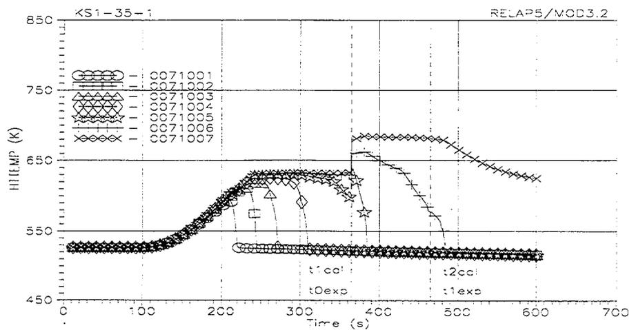
Fig. C-1. RELAP5/MOD3.2-calculated TW(t) heated tube inside wall temperatures histories in the upper, middle and bottom parts of the FA model (tcal=0-600 s). Maximum time step =0.01 s. Restart time t=365 s.
