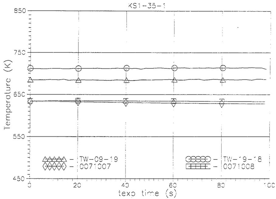
Fig. B-22. Comparison of measured TW19-18(t), TW09-19(t) and RELAP5/MOD3.2-calculated heated tube inside wall temperatures histories in the bottom part of FA model (texp=0-100 s).
