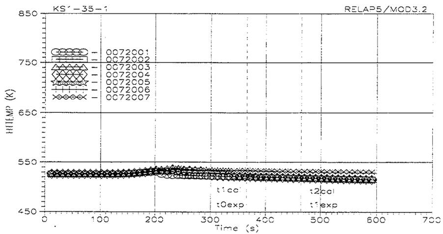
Fig. B-10. RELAP5/MOD3.2-calculated  $T_i(t)$  insulator inside wall temperatures histories in the upper, middle and bottom parts of the FA model ( $t_{cal}=0-600$  s).
