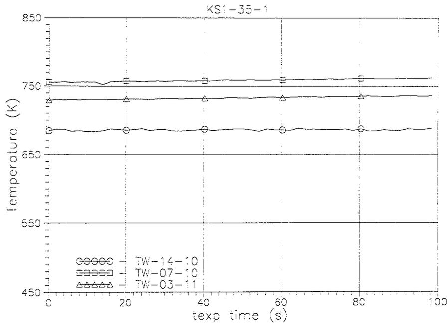
Fig. A-11. Measured TW14-10(t), TW07-10(t) and TW03-11(t) heated tube inside wall temperatures histories in the middle part of the FA model (texp=0-100 s).
