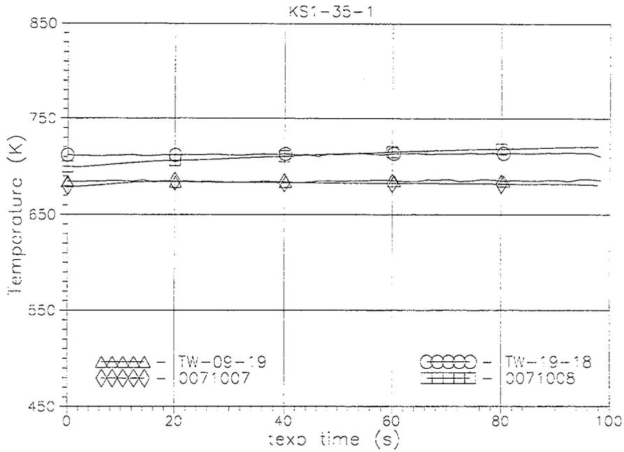
Fig. C-11. Comparison of measured TW19-18(t), TW09-19(t) and RELAP5/MOD3.2-calculated heated tube inside wall temperatures histories in the bottom part of FA model (texp=0-100 s)
