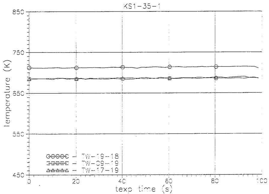
Fig. A-14. Measured TW19-18(t), TW09-19(t) and TW17-19(t) heated tube inside wall temperatures histories in the bottom part of the FA model (texp=0-100 s).
