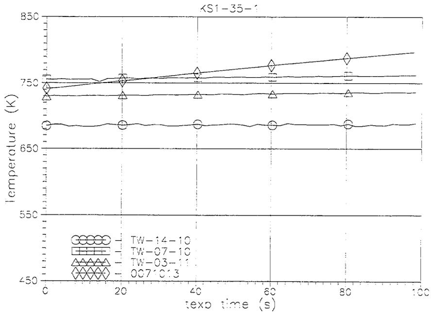
Fig. C-8. Comparison of measured TW14-10(t), TW07-10(t), TW03-11(t) and RELAP5/MOD3.2-calculated heated tube inside wall temperatures histories in the middle part of FA model (texp=0-100 s)
