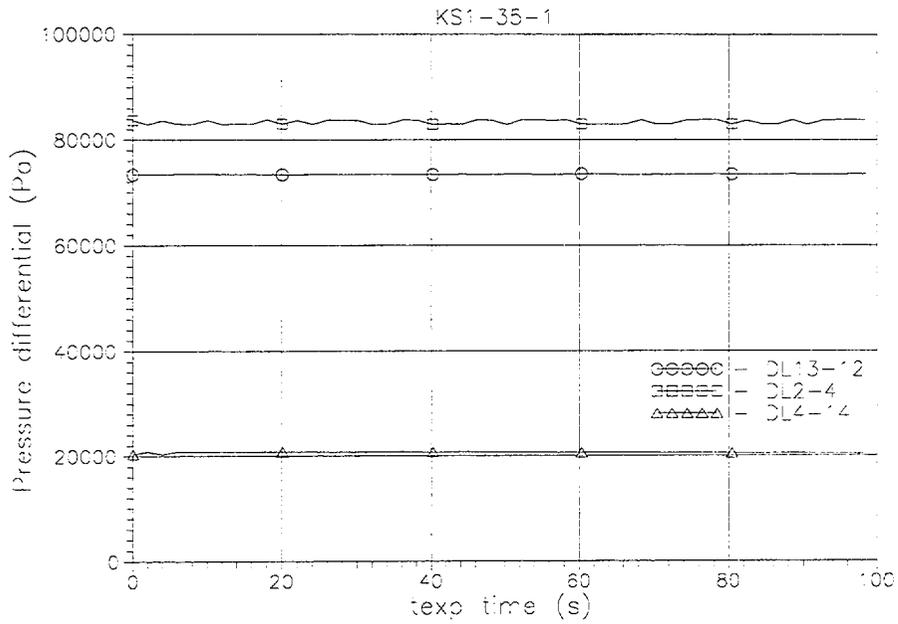
Fig. A-5. Measured DL13-12(t) UP model, DL2-4(t) and DL4-14(t) DC model differential pressure histories (texp=0-100 s).
