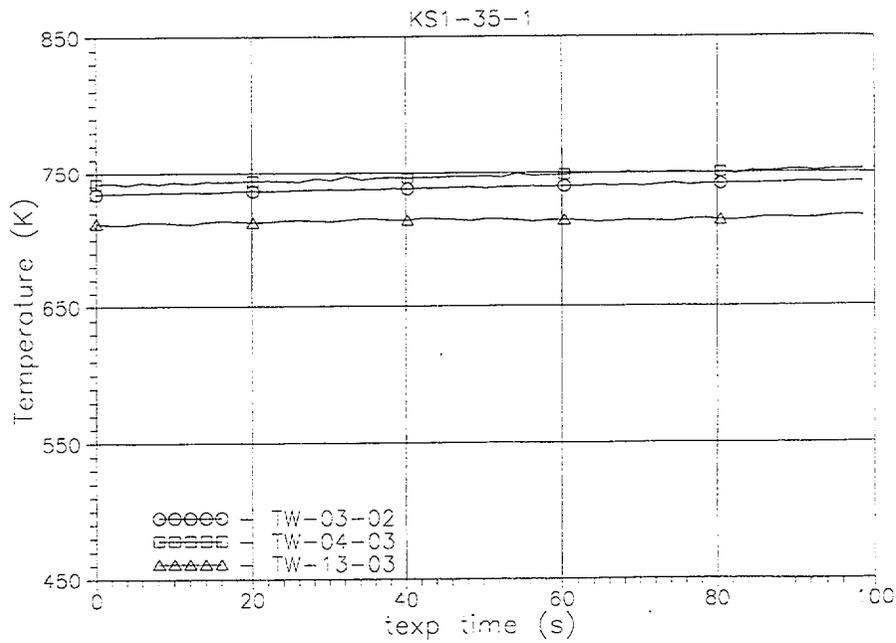
Fig. A-8. Measured TW03-02(t), TW04-03(t) and TW13-03(t) heated tube inside wall temperatures histories in the upper part of the FA model (texp=0-100 s).
