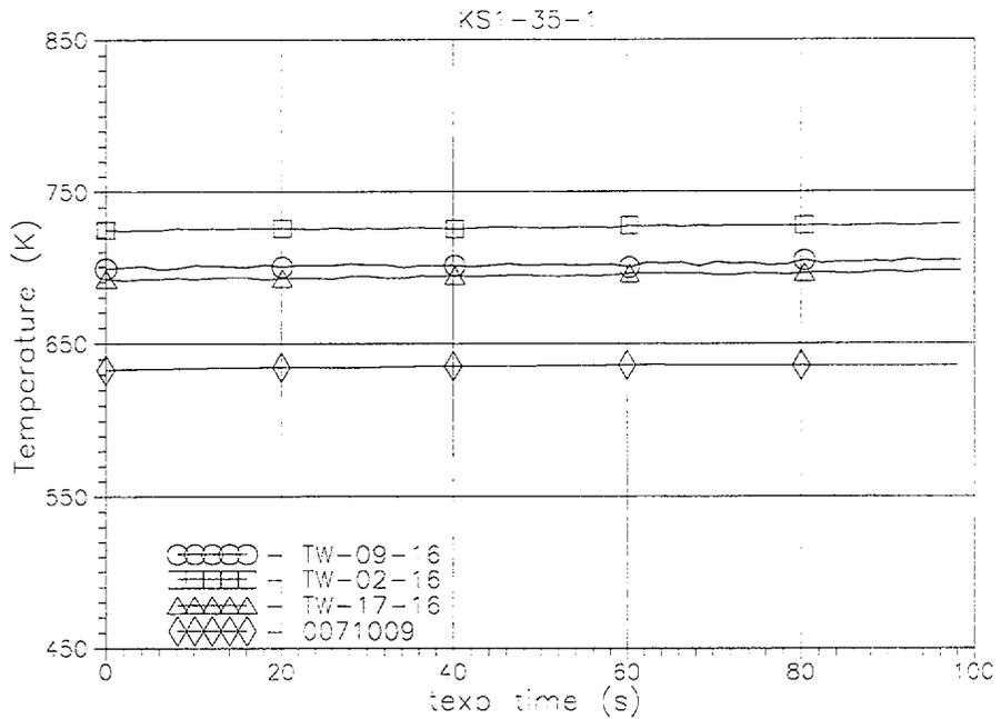
Fig. B-21. Comparison of measured TW09-16(t), TW02-16(t), TW17-16(t) and RELAP5/MOD3.2-calculated heated tube inside wall temperatures histories in the middle part of FA model (texp=0-100 s).
