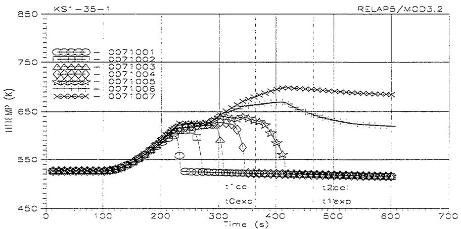
Fig. 5.2. The effect of maximum user-specified time step on the calculated inside wall temperatures histories in the upper, middle and bottom parts of the bundle heated tube ( $t_{cal}=0-600$  s), and also selection of time interval, corresponding  $Dt_{exp}$ , and selection of time moment  $t1_{cal}$ , corresponding  $t0_{exp}$  for KS-1 Test.  $dt_{max}=0.2$  s.
