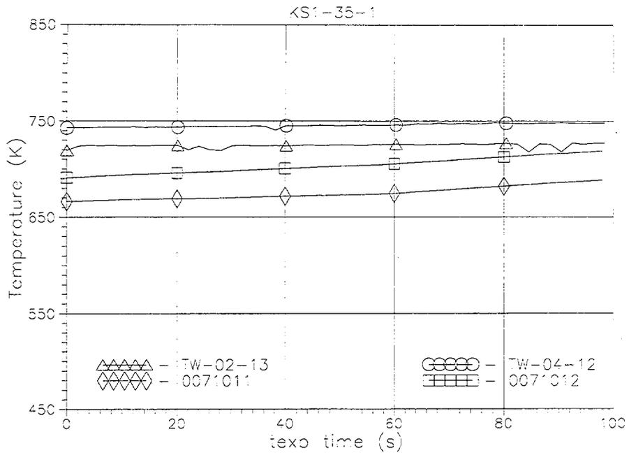
Fig. B-20. Comparison of measured TW04-12(t), TW02-13(t) and RELAP5/MOD3.2-calculated heated tube inside wall temperatures histories in the middle part of FA model (texp=0-100 s).
