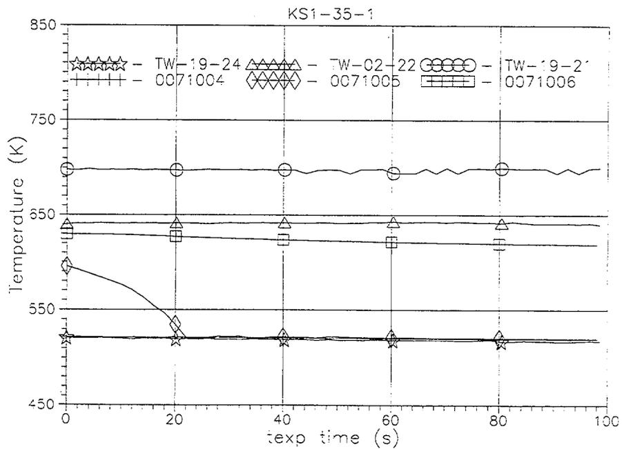
Fig. 4.7. Comparison of measured and RELAP5/MOD3.2-calculated heated tube inside wall temperatures histories in the bottom part of FA Model and also selection of time interval, corresponding  $Dt_{exp}$ , and selection of time moment  $t_{1cal}$ , corresponding  $t_{0exp}$  for KS-1 Test.
