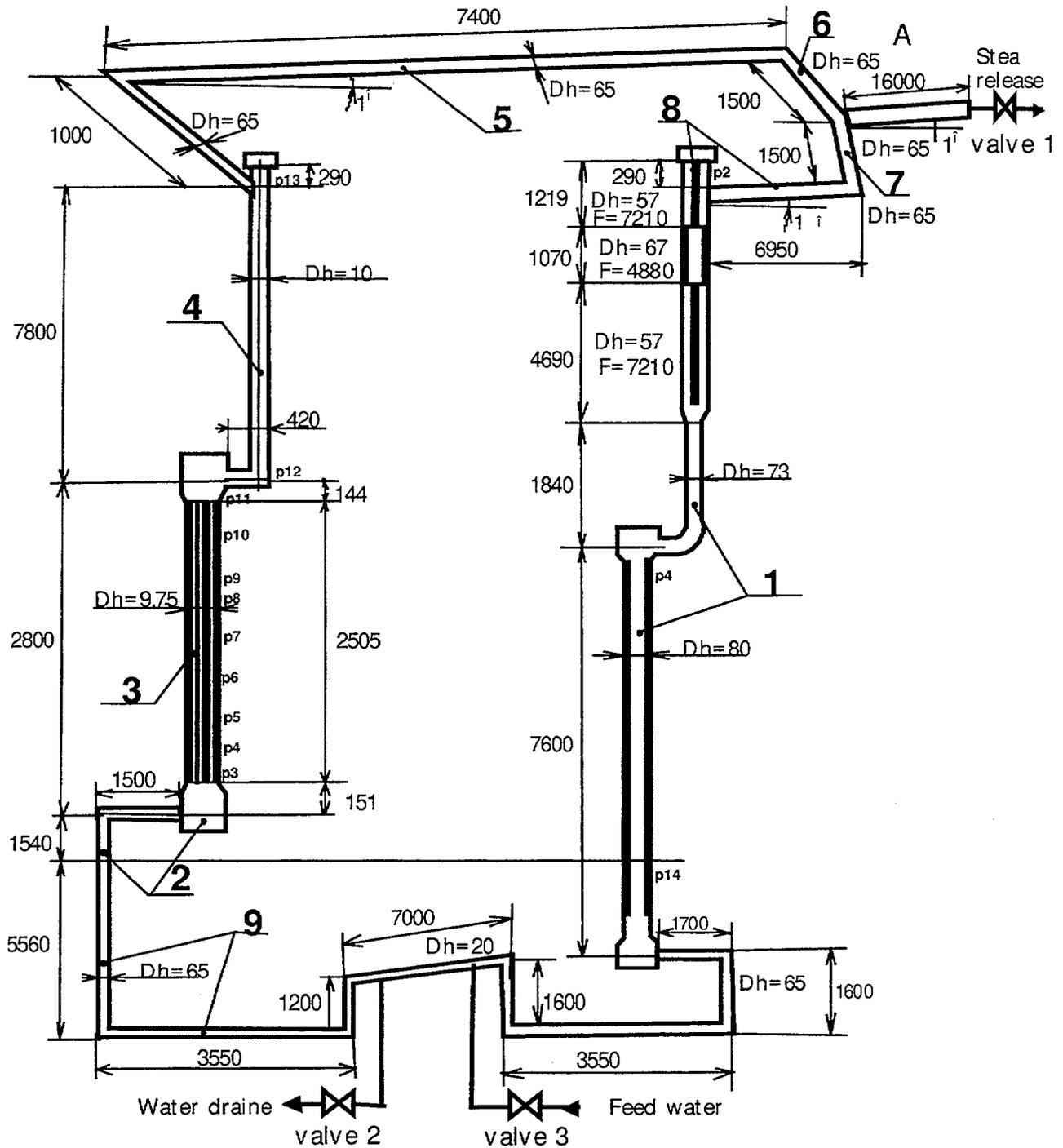
Fig.2.1. Scheme of KS-1 VVER Loop model.
