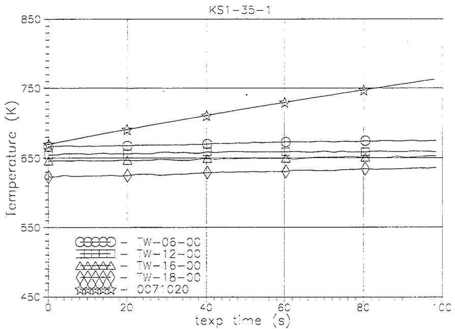
Fig. C-4. Comparison of measured  $TW06-00(t)$ ,  $TW12-00(t)$ ,  $TW16-00(t)$ ,  $TW18-00(t)$  and RELAP5/MOD3.2-calculated heated tube inside wall temperatures histories at the top of FA model ( $t_{exp}=0-100$  s).
