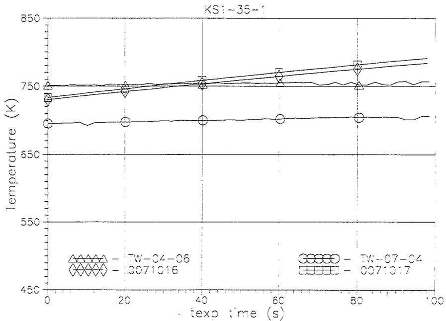
Fig. B-17. Comparison of measured TW07-04(t), TW04-06(t) and RELAP5/MOD3.2-calculated heated tube inside wall temperatures histories in the upper part of FA model (texp=0-100 s).
