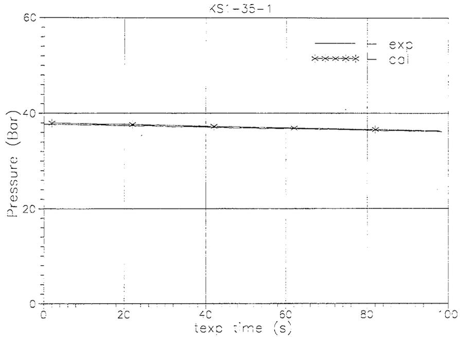
Fig. C-3. Comparison of measured  $P_{out}(t)_{exp}$  and RELAP5/MOD3.2-calculated  $P_{out}(t)_{cal}$  pressure at Core model outlet ( $t_{exp}=0-100$  s).
