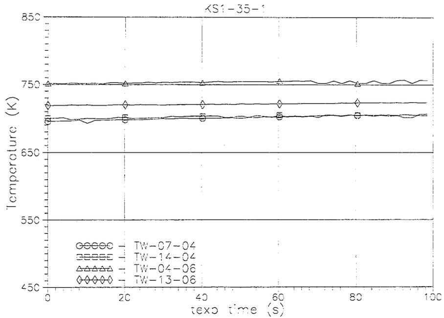
Fig. A-9. Measured TW07-04(t), TW14-04(t), TW04-06(t) and TW13-06(t) heated tube inside wall temperatures histories in the upper part of the FA model (texp=0-100 s).
