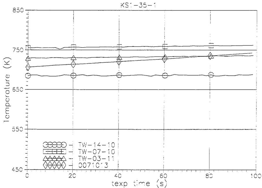
Fig. B-19. Comparison of measured TW14-10(t), TW07-10(t), TW03-11(t) and RELAP5/MOD3.2-calculated heated tube inside wall temperatures histories in the middle part of FA model (texp=0-100 s).
