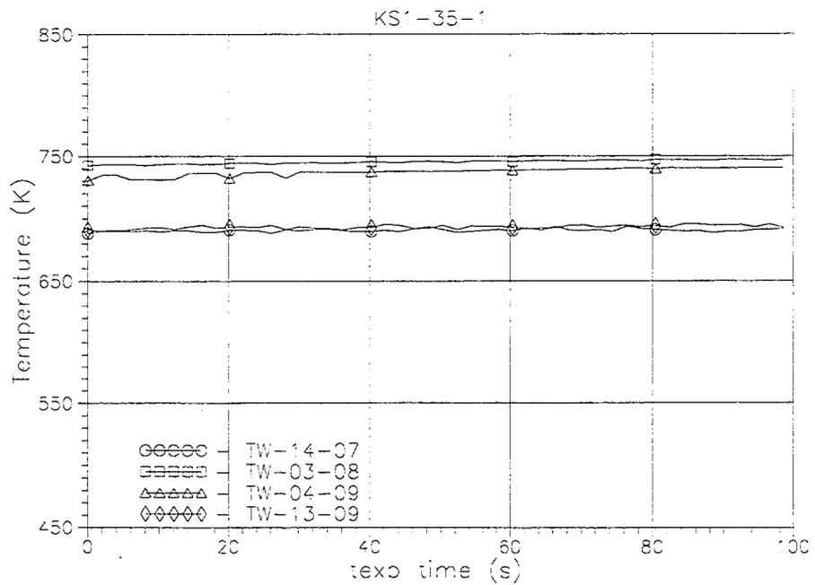
Fig. A-10. Measured TW14-07(t), TW03-08(t), TW04-09 (t) and TW13-09(t) heated tube inside wall temperatures histories in the upper part of the FA model (texp=0-100 s).
