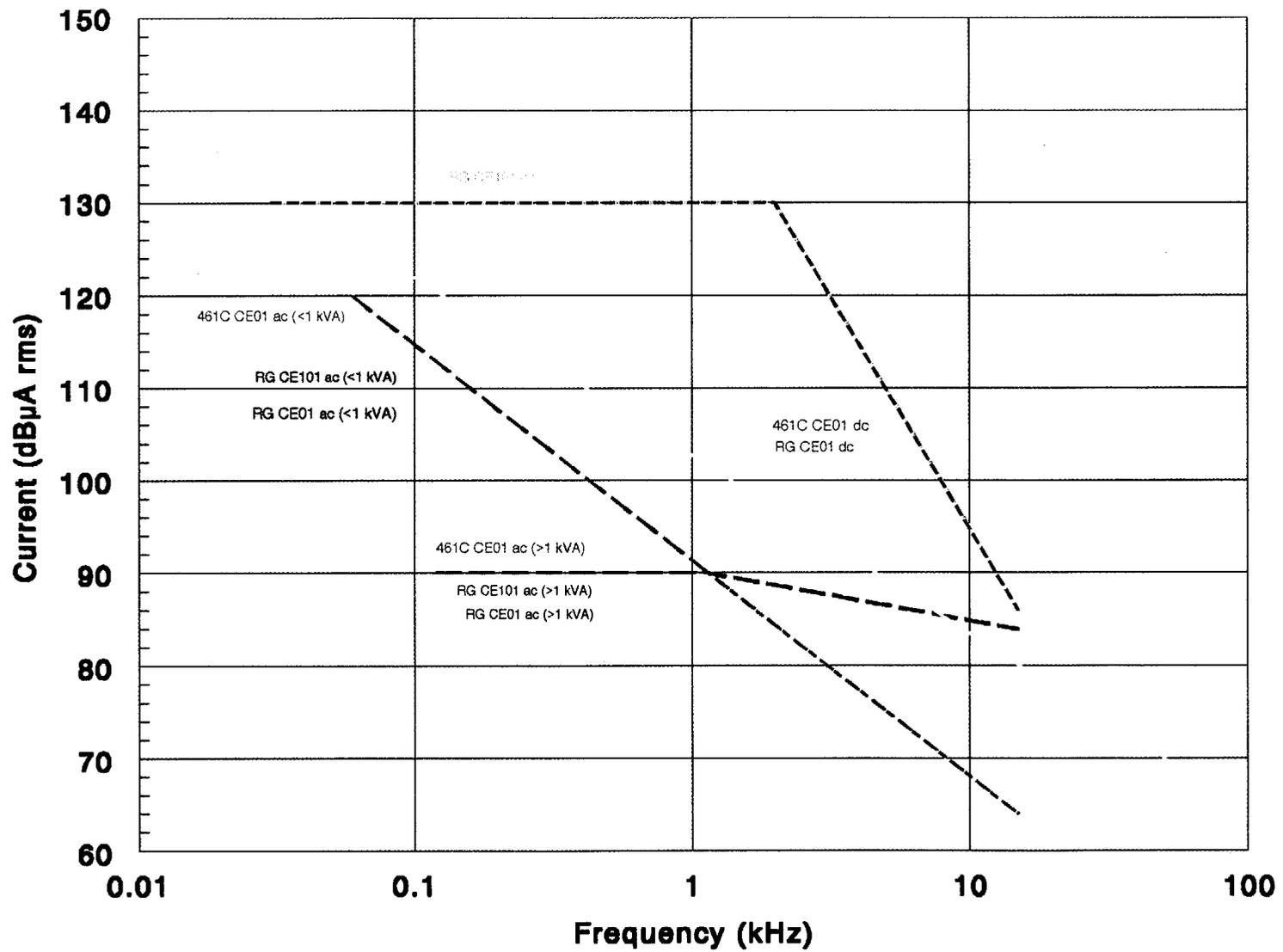
Figure A.5 Comparison of low-frequency conducted emissions envelopes
