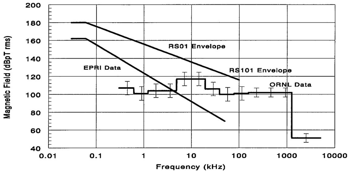
Figure 6.2 Data vs Operating Envelopes, Radiated Magnetic Fields
