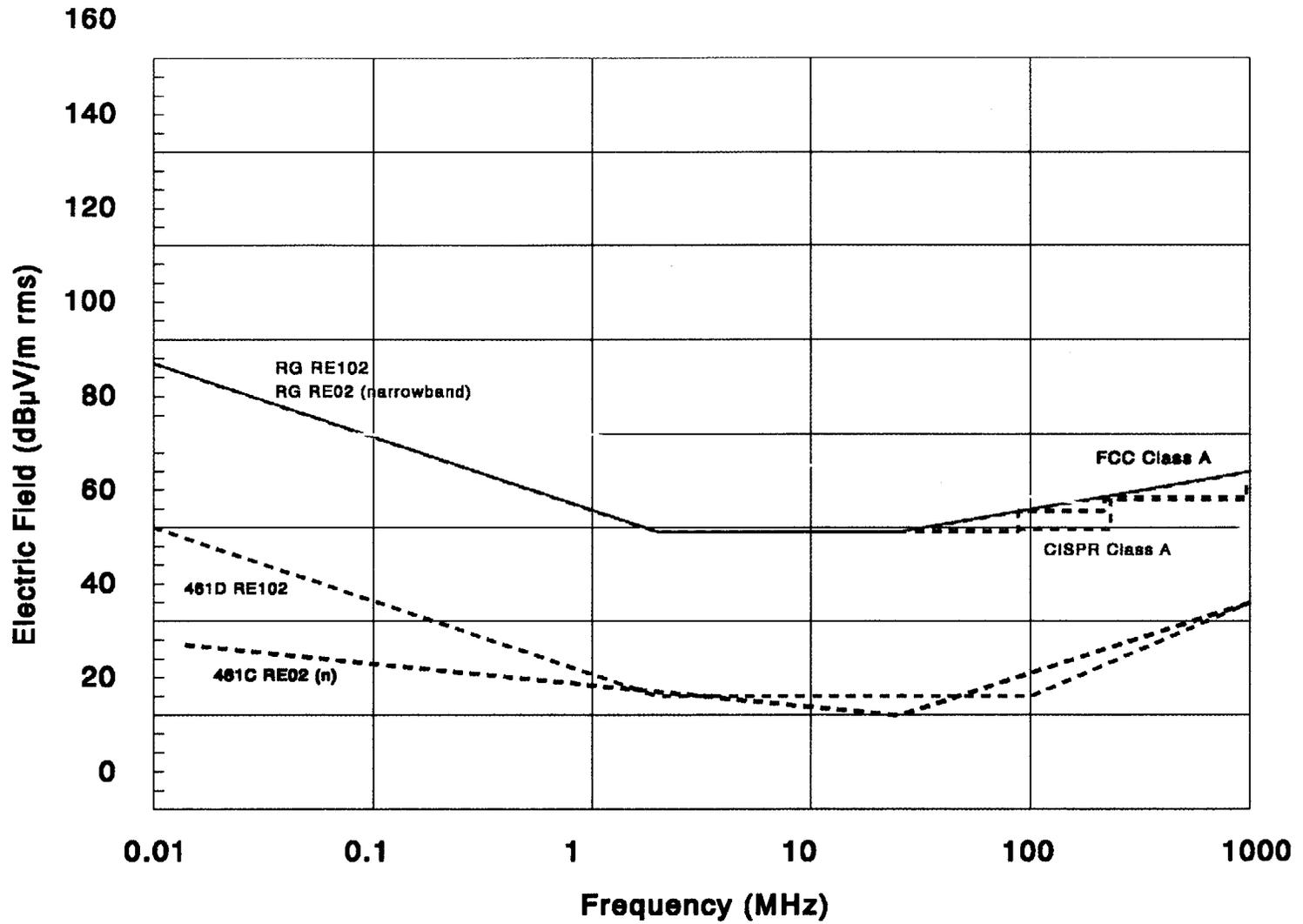
Figure A.8 Comparison of high-frequency radiated emissions envelopes
